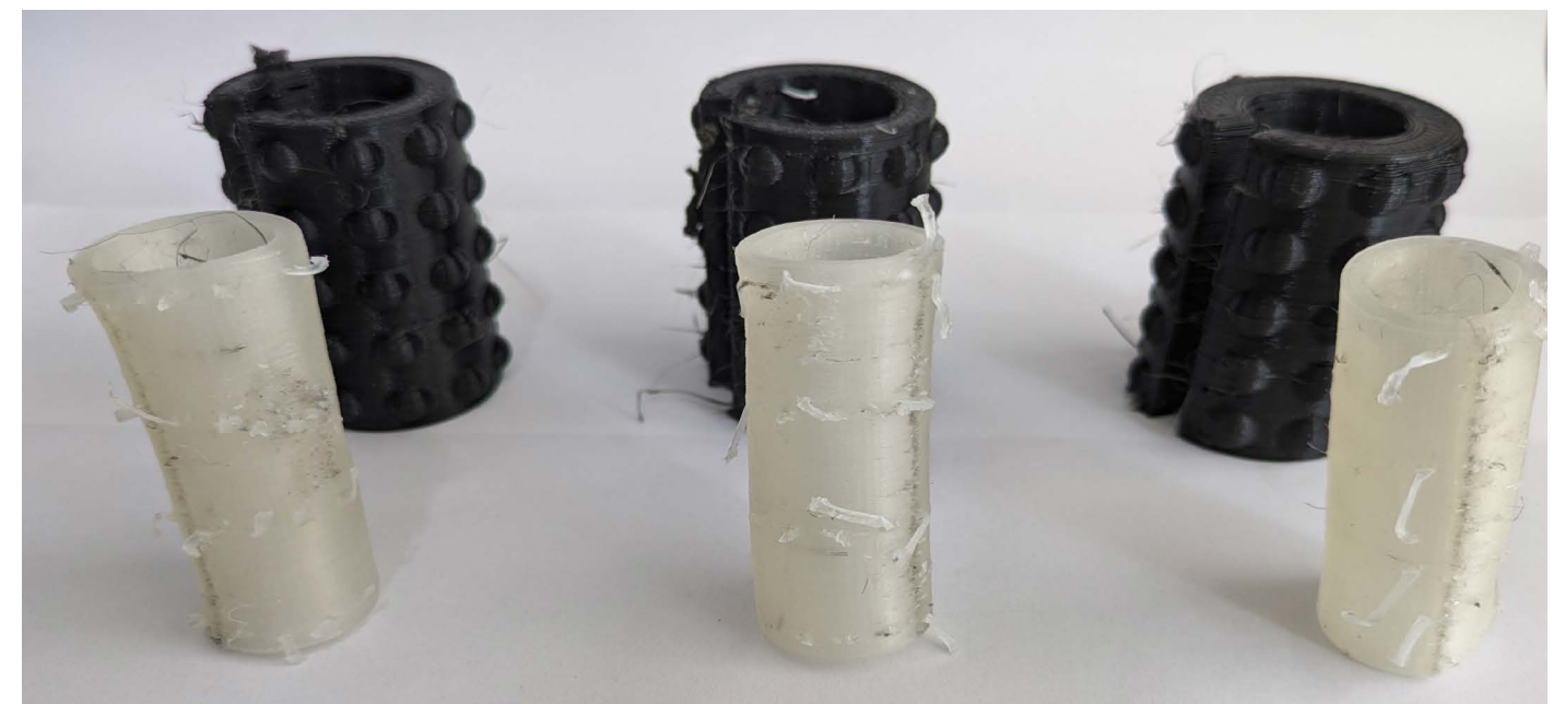
Figure 91: Different designs of thin walls with TPU around PLA. Only connections along seam (left), only connections along seam and low infill for TPU (middle), connections all the way around and thick TPU layer (right)
