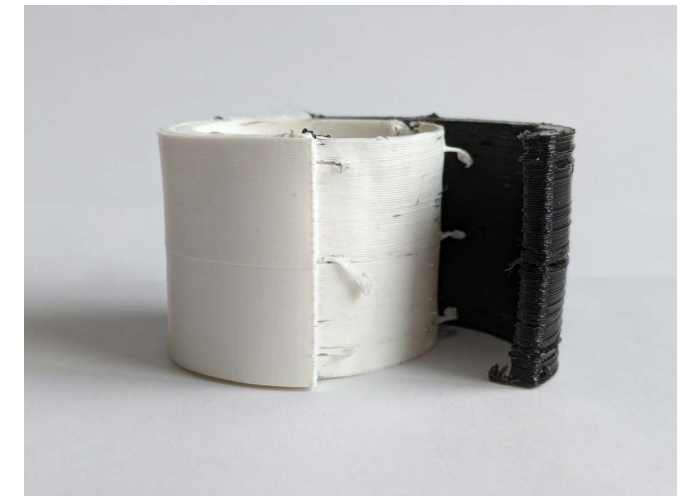
Figure 92: “Peeling” off the TPU from the PLA
