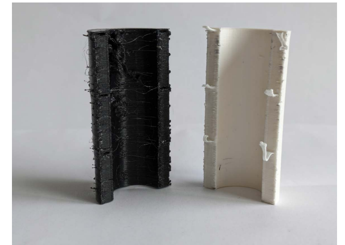
Figure 93: Disconnection of the thin walled handle. A clean separation except for the Z-seam overextrusion contamination
