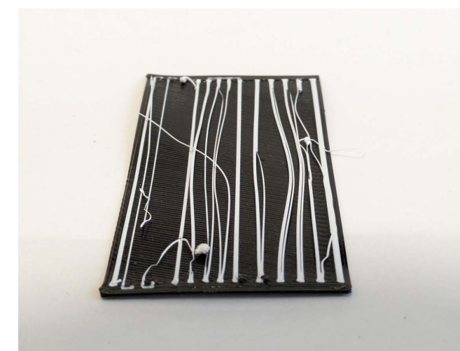
Figure 29: Testing the different speeds at which PLA will still adhere to the TPU
