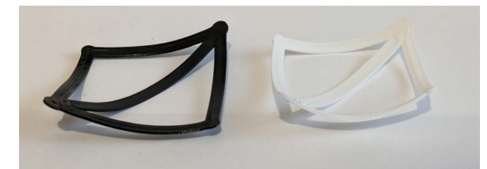
Figure 27: Testing folding in different directions at the same time
