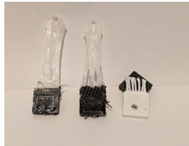
Figure 77: The alternating layer method (left), the hacksaw method (middle) and the proposed Z-pin method (right)
