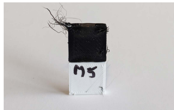
Figure 46: An example of the stringing of the TPU
