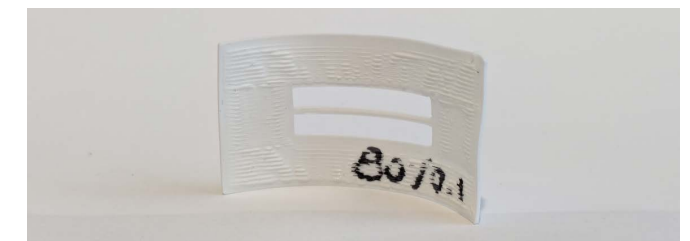
Figure 26: Testing if the shrink force was strong enough to detach a thin piece of PLA, which it was not.
