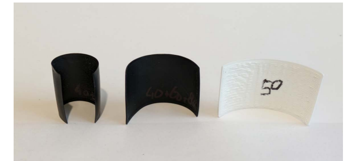
Figure 25: Testing the folding and bending of thin PLA samples with different printing speeds
