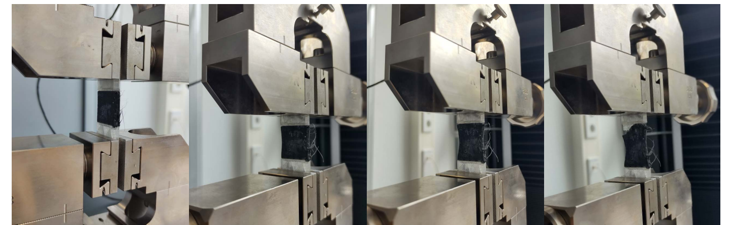
Figure 72: The process of necking and slipping at one of the short edges
