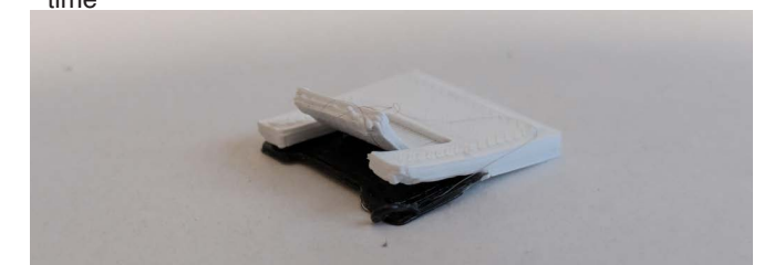
Figure 28: Verifying that the PLA can be detached from the TPU with the SM effect.
