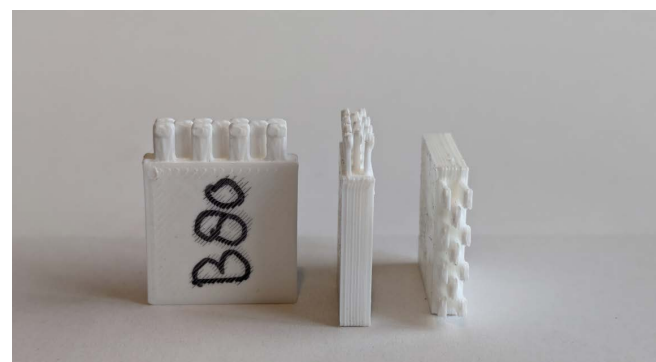
Figure 68: Close up of Z-pin after tensile test
