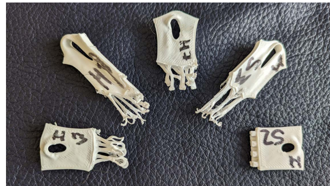
Figure 43: Heated release samples without a trace of TPU contamination
