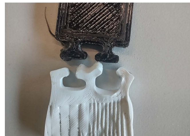
Figure 31: Disconnecting heated PLA from TPU
