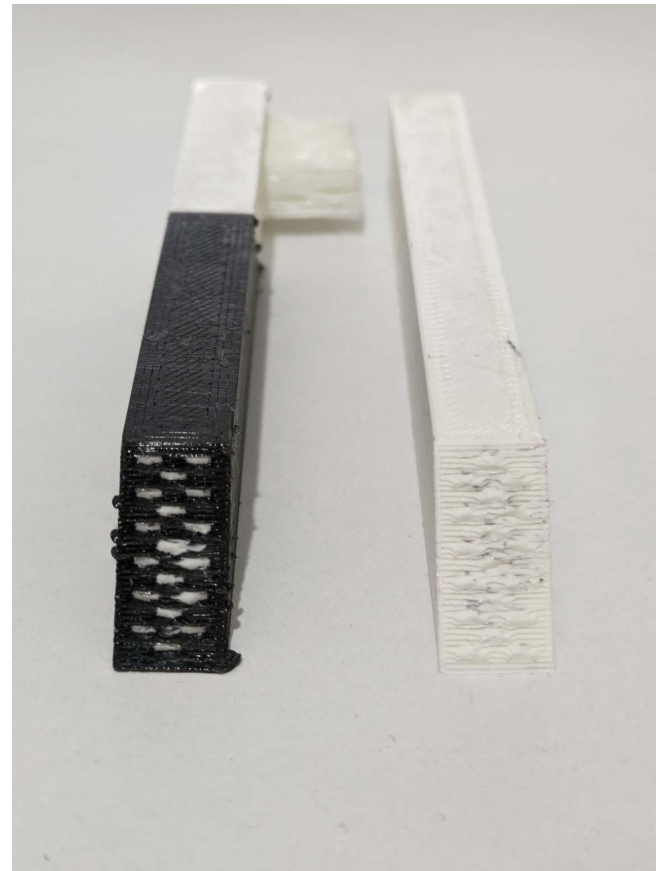
Figure 85: The connective elements break more easily due to the acute angle, which increases stress concentrations
