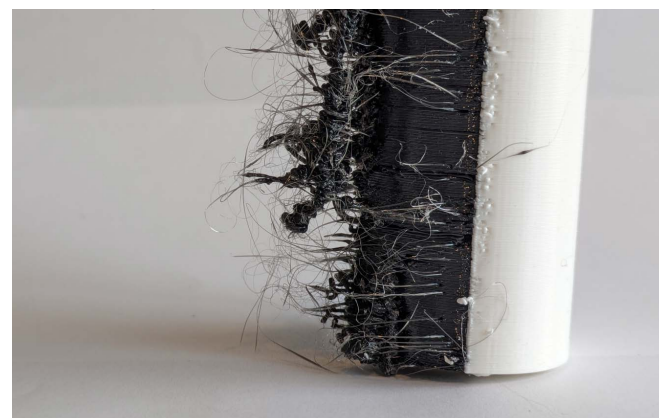
Figure 45: Extreme case of oozing and stringing of the TPU
