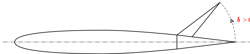
Figure 3.14: Definition of Positive Pitch Deflection.
