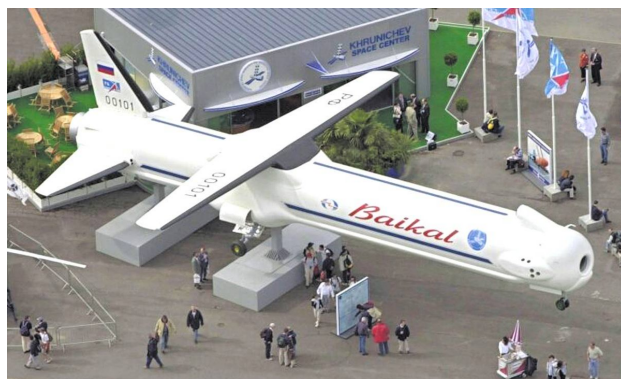
(a) Full-Scale Engineering Model of the Baikal Fly-Back (FB) Booster at the Salon du Bourget (Paris Air Show) 2001 [171].
