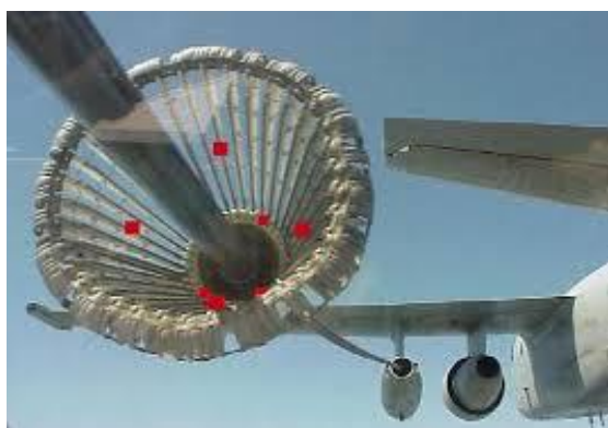
Fig. 2: Aerial refuelling drogue with VisNav beacons and boom from the receiver aircraft [36]
