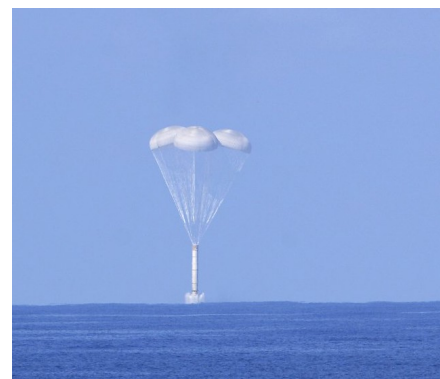
(b) Splashdown of a Space Shuttle Solid Rocket Booster (SRB) after STS-124 [172].
