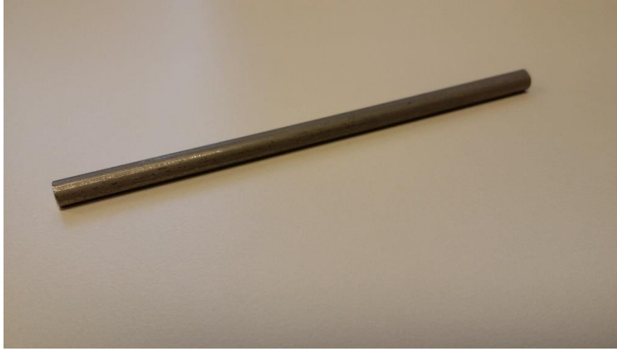
Figure 3.1: The pipe phantom used in the rolling shutter effect measurements.
