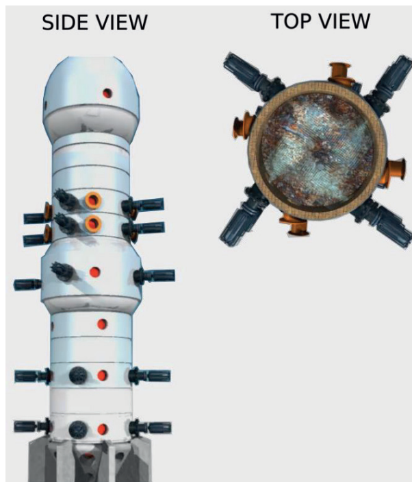
Fig. 5.3. Schematic representation of multiple microwave generators attached to a single reactor [23]. Note that each of the black elements represents a 20 kW microwave plasmatron.
