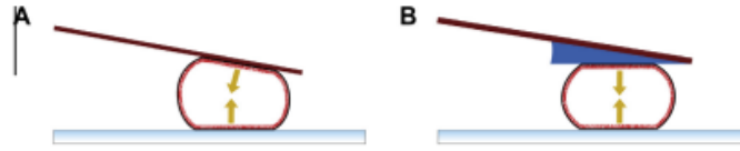
Figure 3.4: An image of a cantilever pushing on a cell without a wedge (A) and a cantilever with a wedge (B), in the cantilever with a wedge the forces align better and there will be less lateral displacement of the cell [63]
