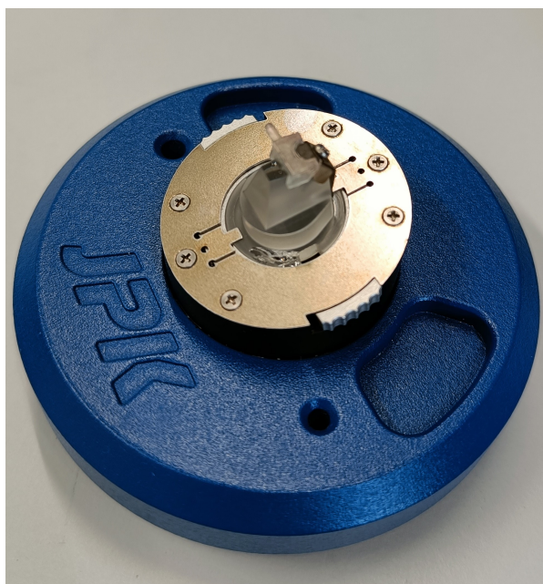
Figure A.3: A cantilever mounted on the JPK cantilever holder
