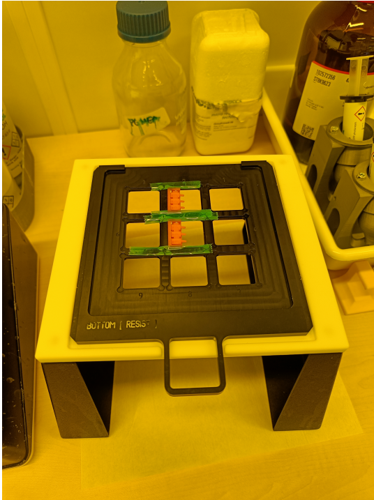
(a) Fluid interfaces mounted in the Nanoscribe sample holder, ready for printing.
