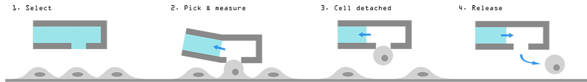
Figure 2.6: A schematic representation of FLuidFM [52]
