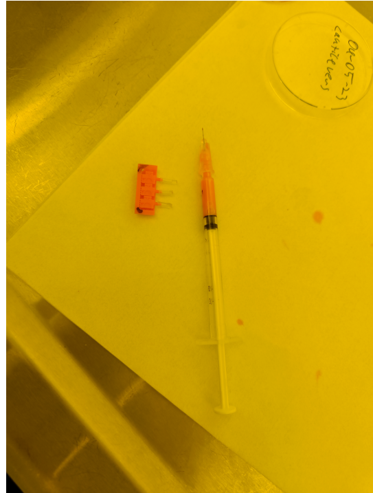
(b) FLuid interfaces plugged and the exit holes filled with a droplet of resin, the resin is applied with the syringe.
