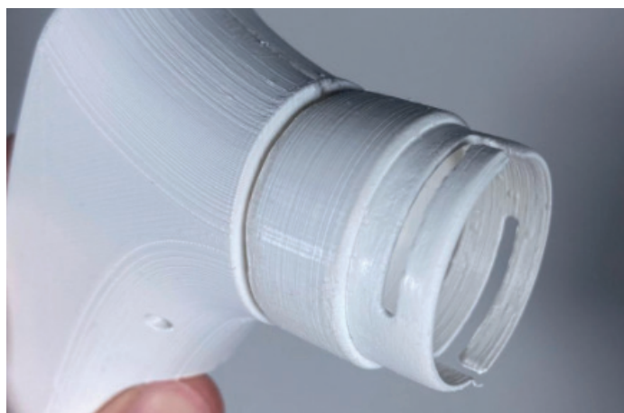
Figure J.35 - Bayonet lock option 2 disassembled static handle
