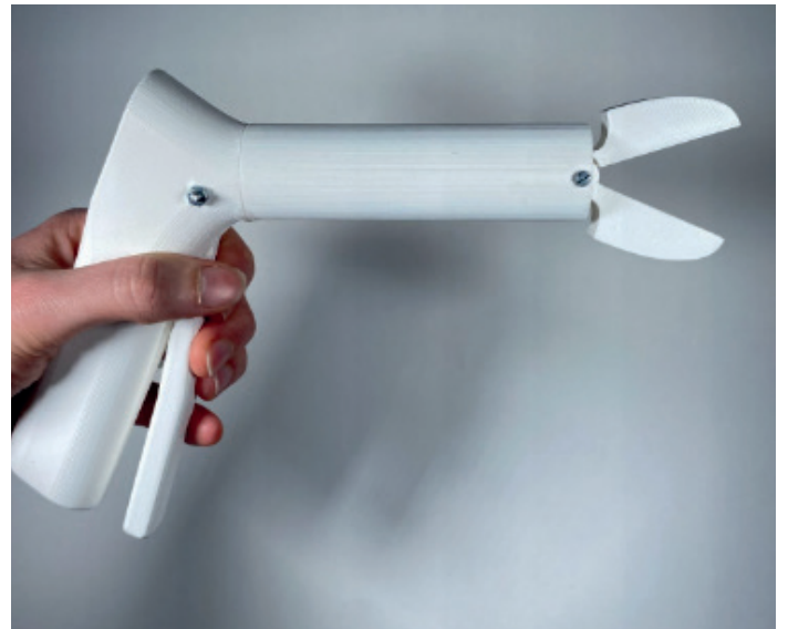
Figure I.13 - Images of the stages of opening of the linear cam mechanism attached to a working handle
