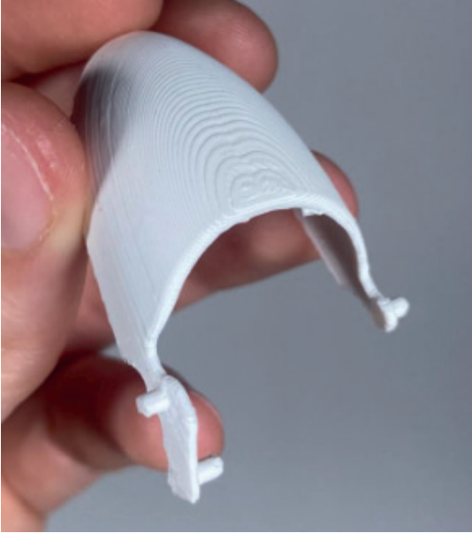
Figure J.22 - Flap iteration using rapid prototyping
