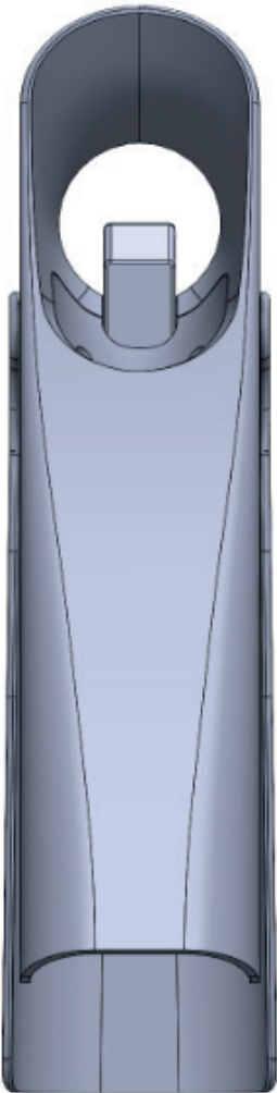
Figure J.29 - Cam obstructs entry to main body when squeeze handle not compressed
