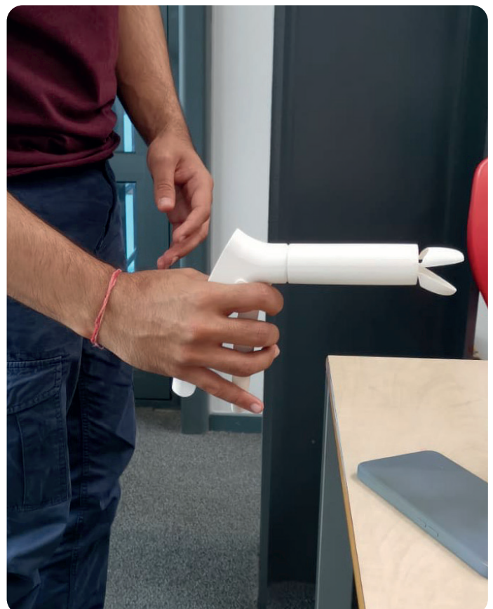
Figure 5.1 - Testing handle ergonomics for the user when the patient bed is lower
