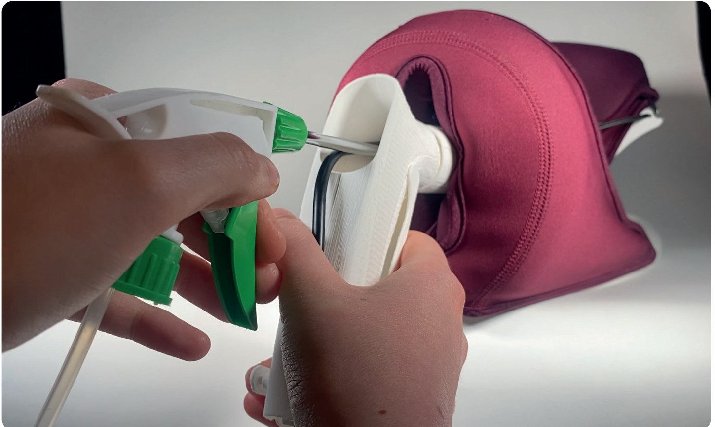
Figure 5.2 - Testing ability to insert apparatus into the narrower inner tube of the C Spec using the Mama U model
