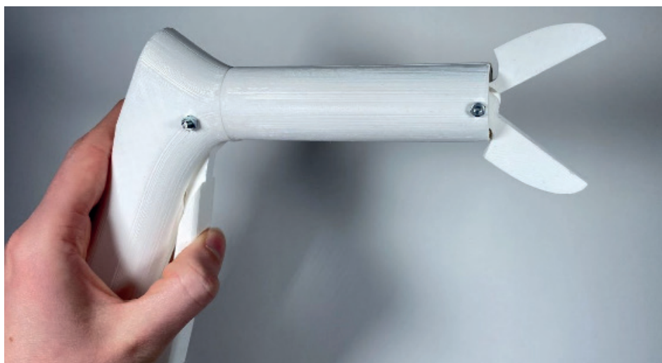
Figure I.18 - Images of the rotating hinge mechanism close up integrated into the handle in an open state
