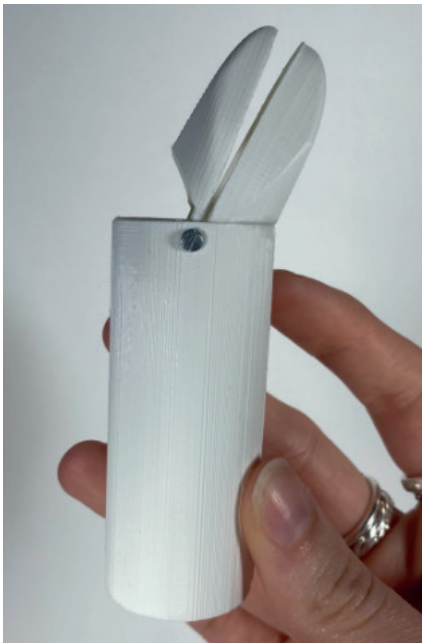
Figure I.20 - Images of the single flap moving mechanism using a linear cam showing the hollow feature
