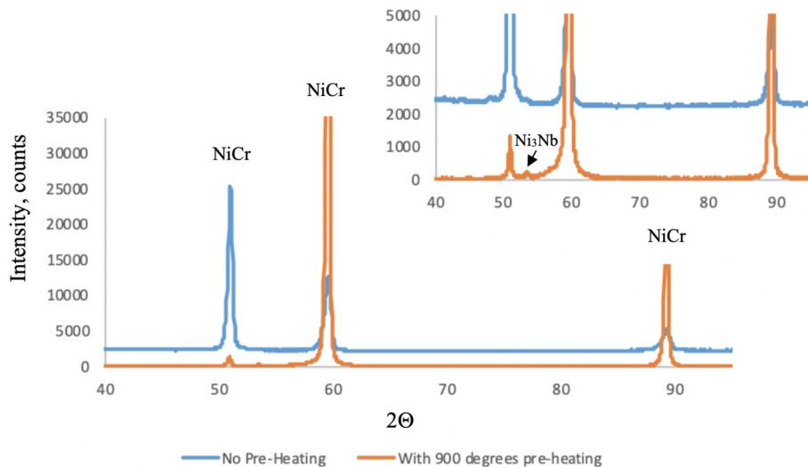
**Fig. 6.** XRD phase composition (including enlarged section), showing comparison between samples built with 100  $\mu\text{m}$  layer thickness, with and without pre-heating.
