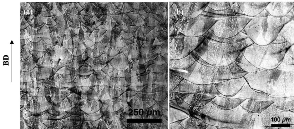
**Fig. 3.** Microstructure of specimens made by SLM with a layer thickness of 50 µm.
