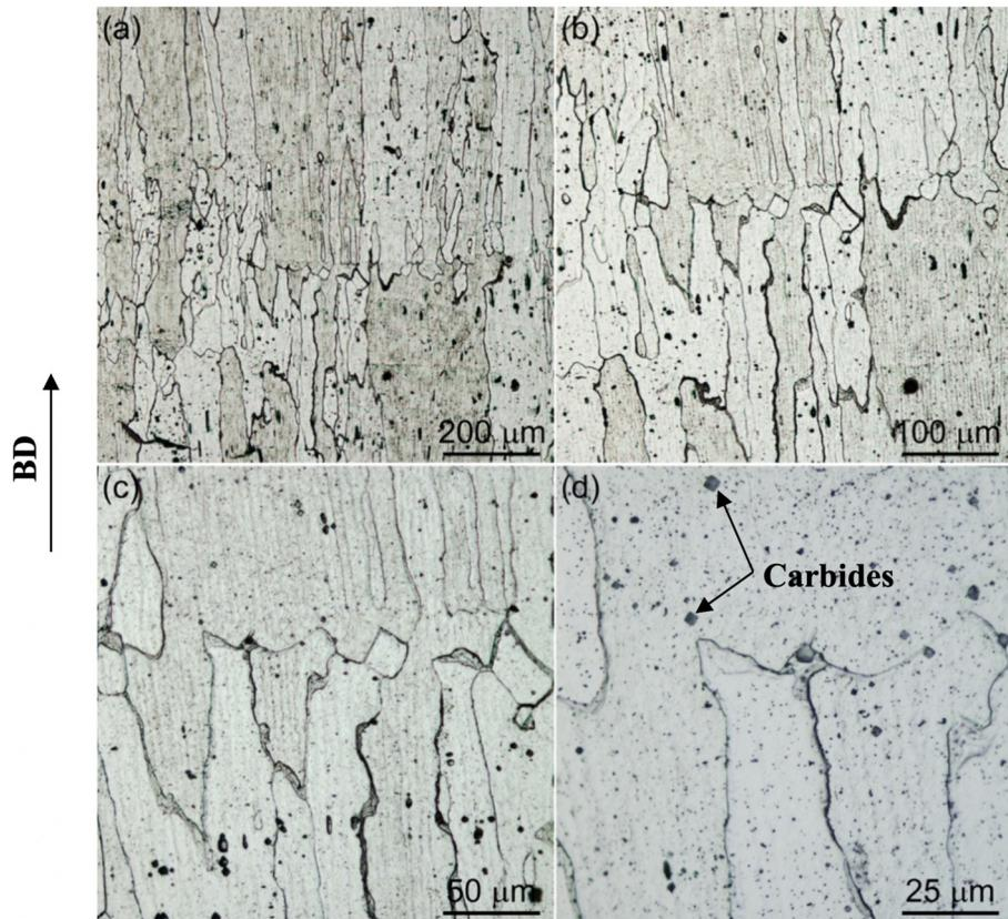
**Fig. 5.** Microstructure of specimen with a layer thickness of 100  $\mu\text{m}$  and 900  $^{\circ}\text{C}$  preheating.
