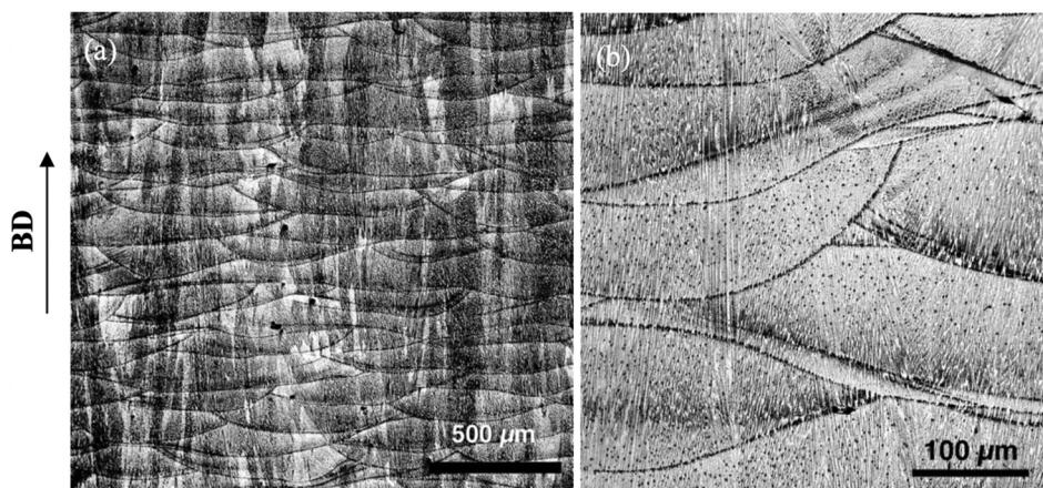
**Fig. 4.** Microstructure of specimens with a layer thickness of 100 µm and without pre-heating.
