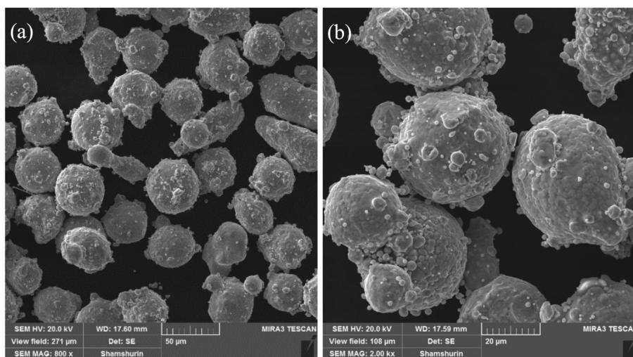
**Fig. 2.** SEM-images of Inconel 718 powder particles.
