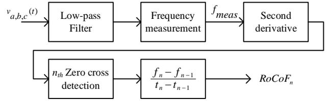
Fig. 2. Block diagram of the Inflection Point Detector.
