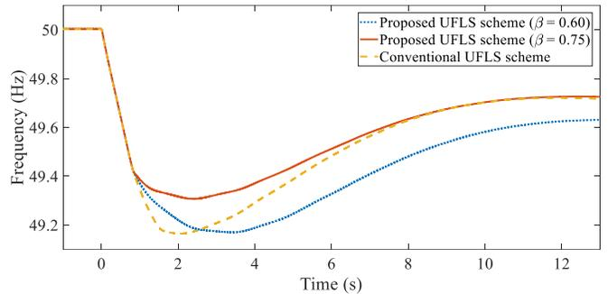
Fig. 12: CoI frequency response using different adjustment coefficients.
