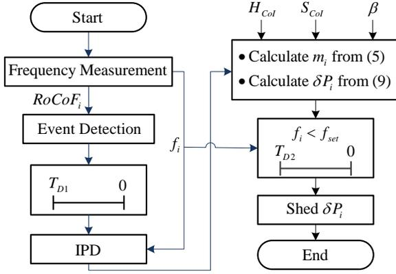
Fig. 3. Flowchart of the proposed UFLS scheme.
