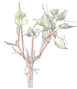
Figure 5: Topology of tree filtered using wood and leaf classification, compared to original point cloud and ground truth in red
