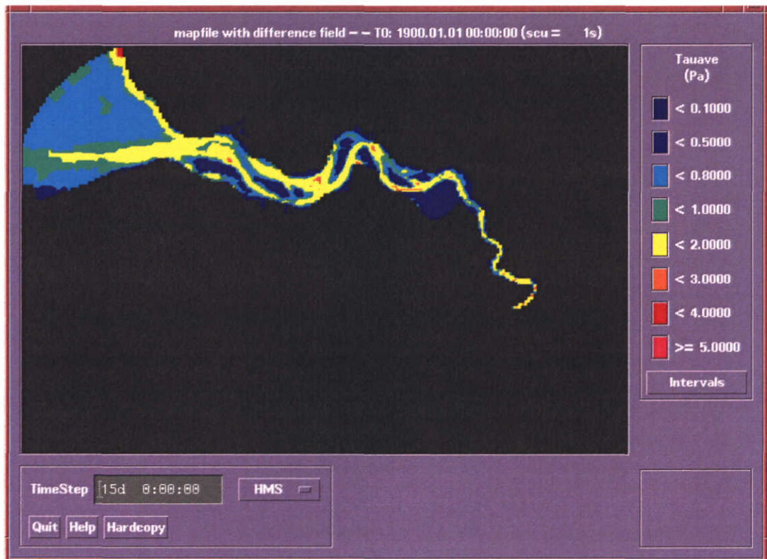
Figure A.6.a The average bed shear stress over 7 model days without wind for the neap period (from day 7-14 of the hydrodynamic data base).
