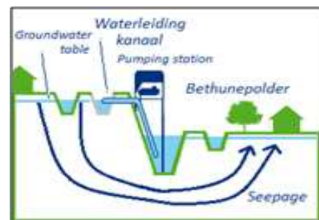
Figure 7-2 Cross section of Bethunepolder
