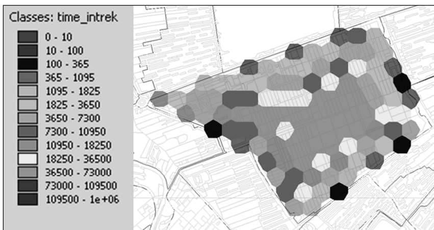
Figure P Residence time of seepage water Bethunepolder [d] (Ministerie van Infrastructuur en Milieu, 2013)
