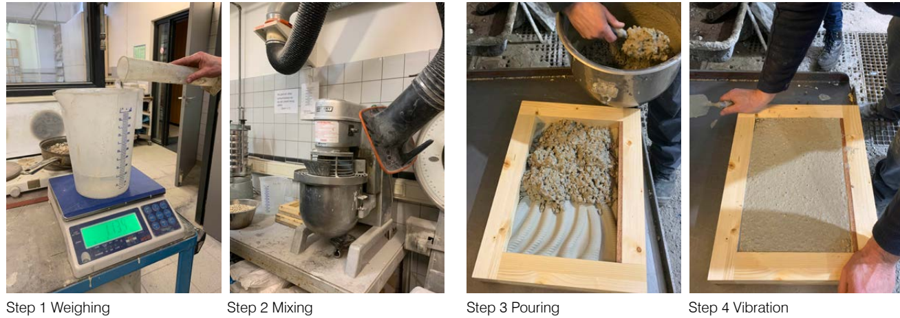
Fig 6.4a: Casting process for concrete panels
