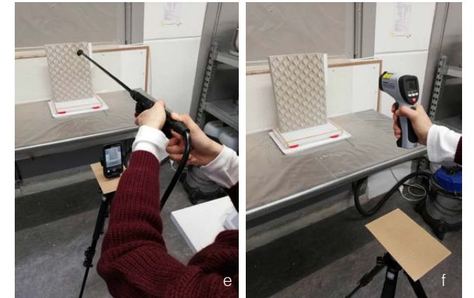
Fig 7.2e, f: e. Water straying, f. Temperature recording
