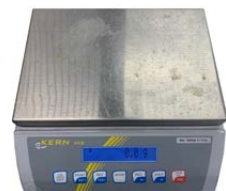
Kern FKB 36K0.1 table scale Use: Weight reading
