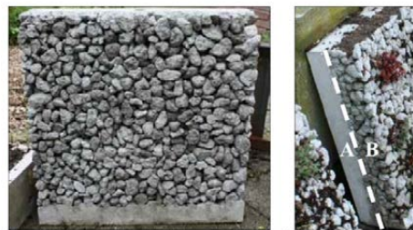
Fig 3.4g: Two-layered concrete block (Ottele, 2010)
