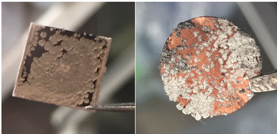
Figure A.5: Comparison of 3\text{mAh}\cdot\text{cm}^{-2} of Li deposited on the 3DPNi (left) and Cu (right) substrate. The homogeneity in the case of 3DPNi is evident.
