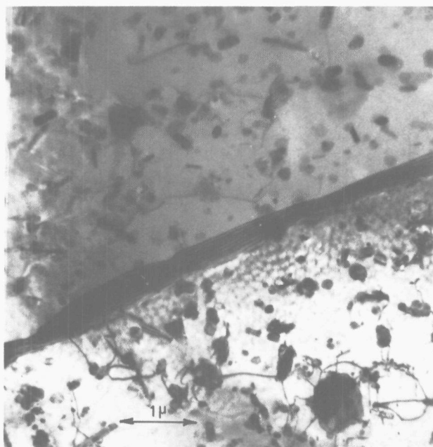
(b) Inclusions of various shapes in 7075 material.
