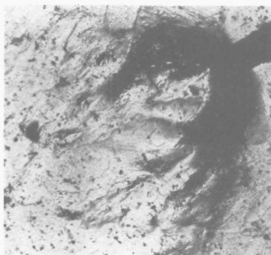
(b) At the onset of crack growth (Note zones of heavy shear deformations).
