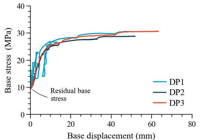
Figure 4: Mobilised base resistance, including residual stresses
