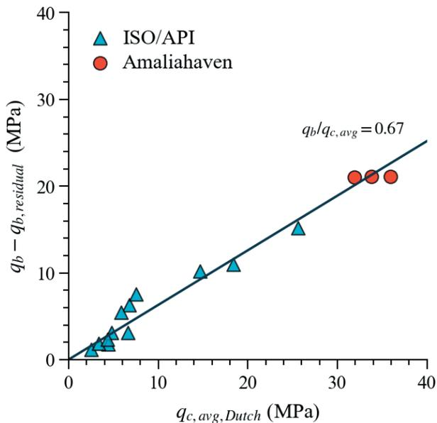
Figure 5: Comparison of the Amaliahaven results with the ISO/API database. The Dutch 4D/8D averaging method was used to determine  $q_{c, avg}$
