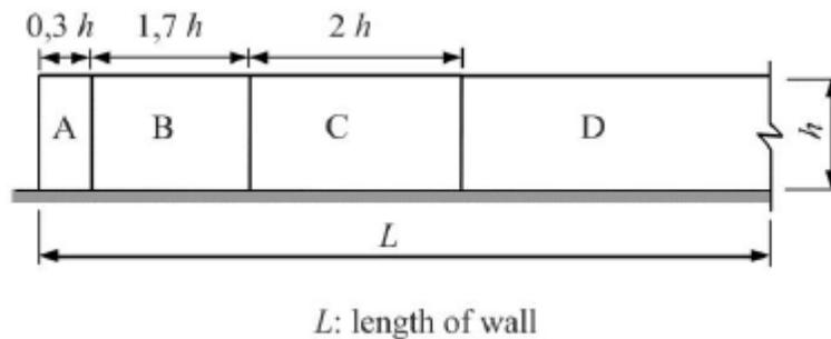
Figure K.2: Zones for free standing walls and parapets with a  $L > 4h$  in accordance with SANS10160-3:2018.
