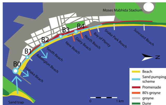
Figure 2.11: A map with the beaches and pumping scheme of Durban . Three of the groyne are constructed in the '80s and are indicated in orange. The groyne at Addington Beach is a pier, not a groyne.
