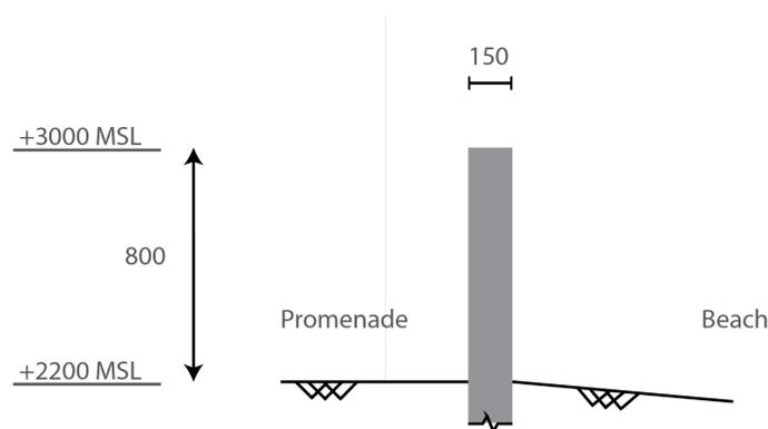
Figure 4.15: A part of the section of the seawall, all measurements are in mm
