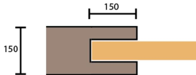
Figure 4.17: An impression of the U-shaped slot, all measurements are in mm
