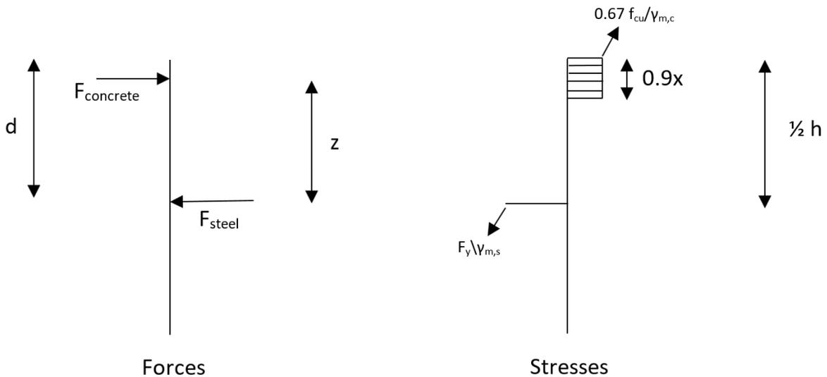
Figure L.3: Sketch of the forces and stresses in the cross-section
