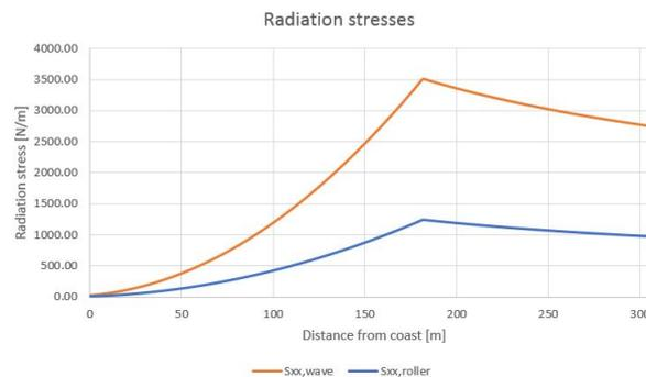
Figure J.2: Radiation stresses of waves and rollers
