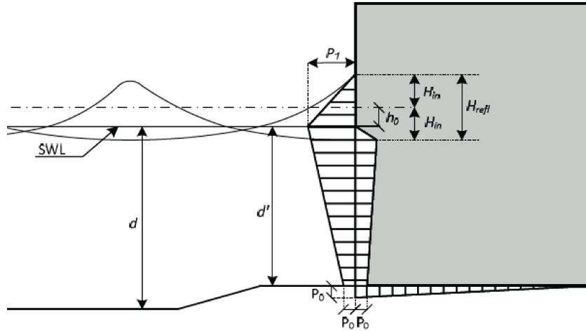
Figure K.3: Sainflou's method to determine forces from waves.[39]
