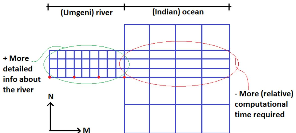
Figure 3.5: Indicative figure about the two grid refinements
