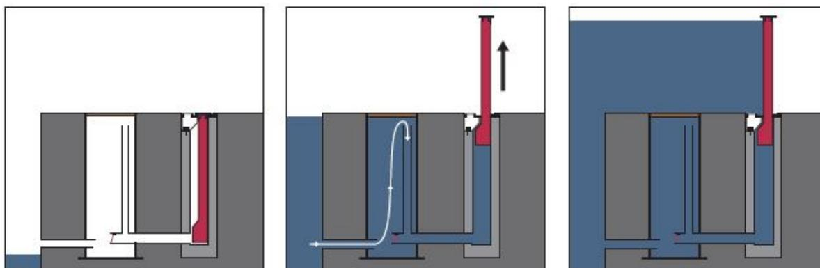
Figure F.5: Illustration of the self-closing barrier
