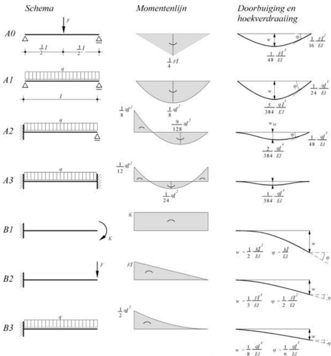
Figure M.1: Engineering formulas for deflection and rotation of a structural element.
