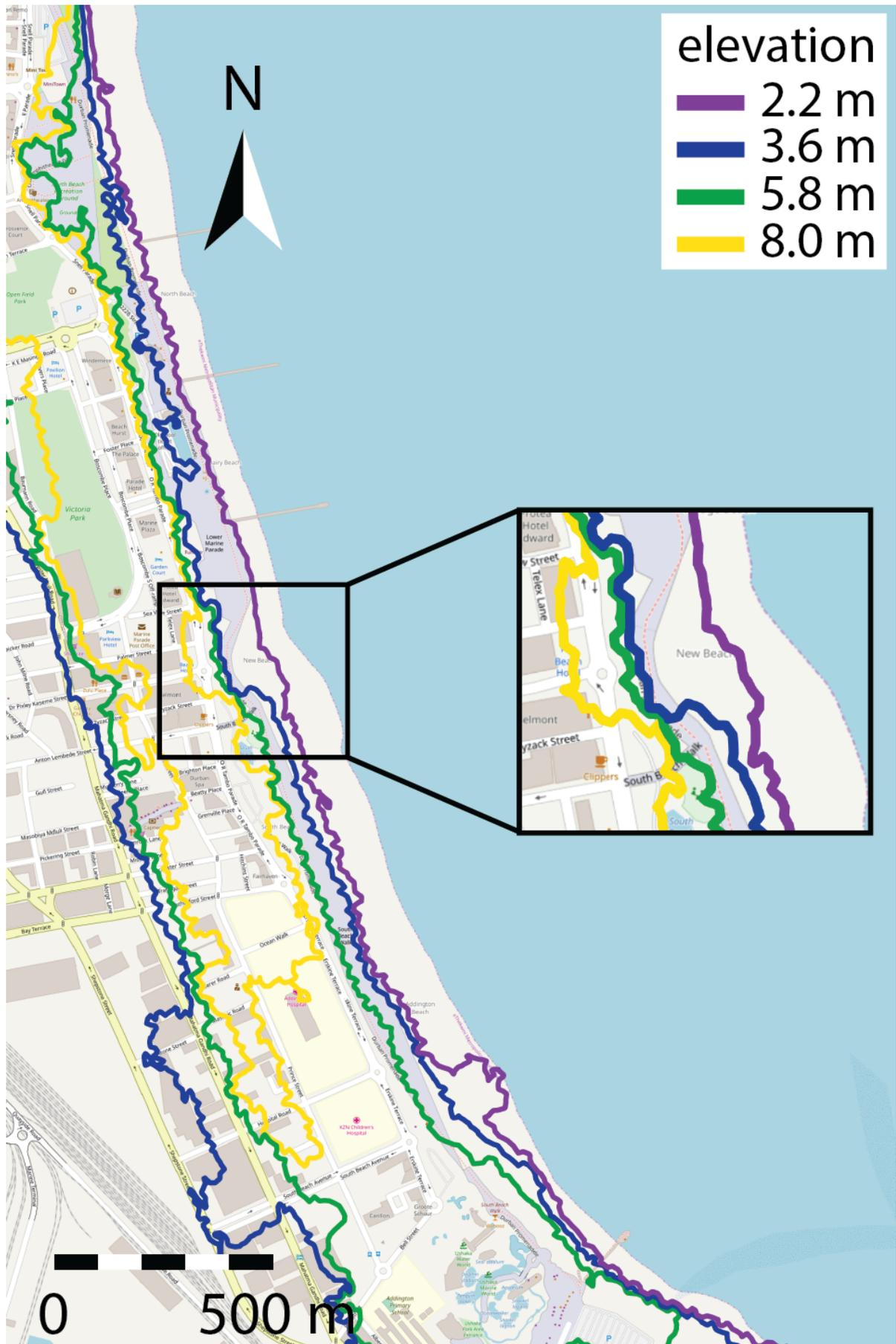
Figure E.2: Elevation of the Durban beachfront relative to the 2016 MSL. The elevation change around New Beach can clearly be seen in this figure.
