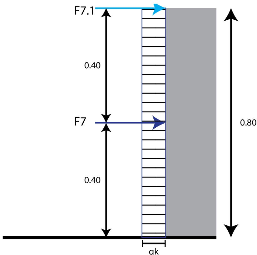
Figure 4.13: Horizontal forces acting on the sea wall due to impact. Distances in meter.
