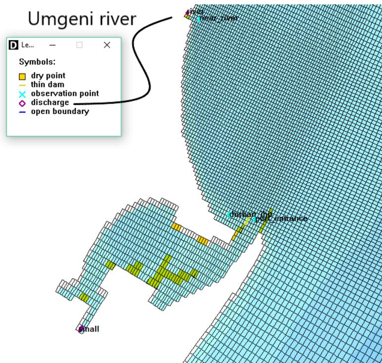
Figure 3.2: The grid of the ocean model in Delft3D, including the boundary condition from the river
