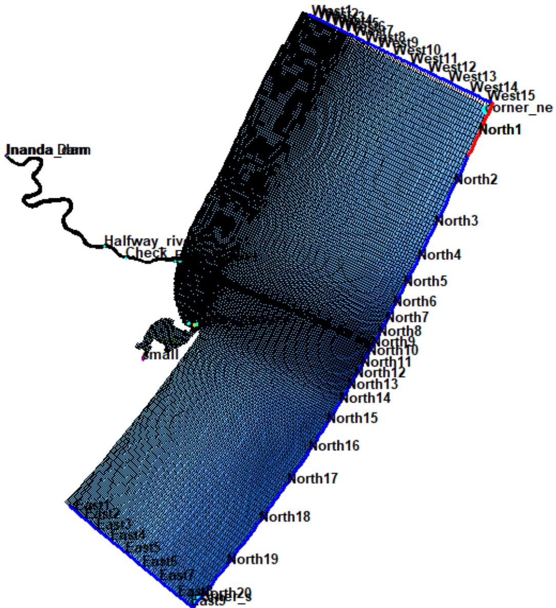
Figure 3.6: The total grid for river and ocean section
