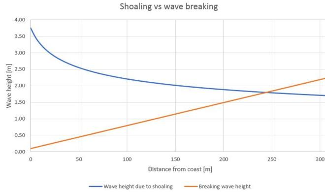
Figure J.1: The shoaling effect and the wave breaking limit visualised
