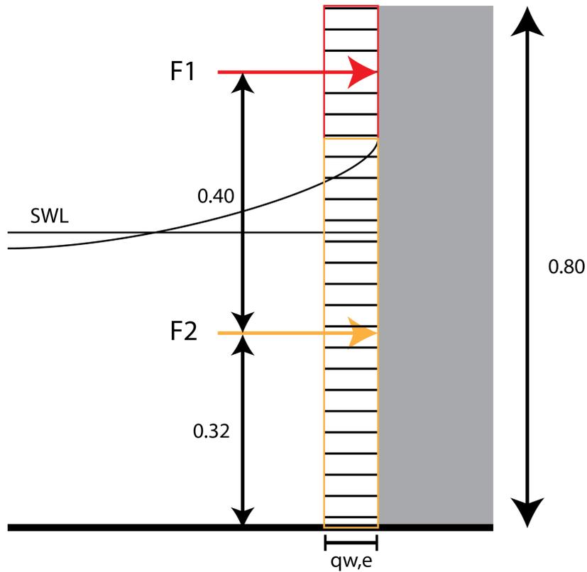
Figure 4.10: Wind pressure on the wall. Distances in meter
