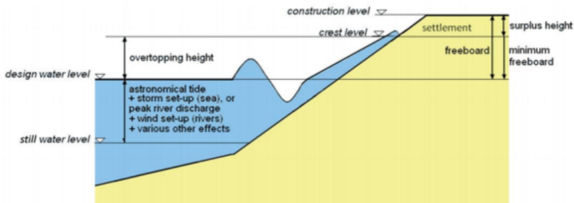
Figure 4.6: Determination of the water-retaining height of the flood defence
