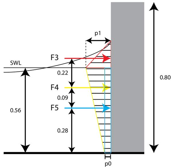
Figure 4.11: Wave induced pressure according to Sainflou's method. Distances in meter.
