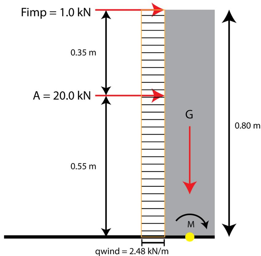
Figure L.1: Governing load combination for both the moment and shear force at ground level.
