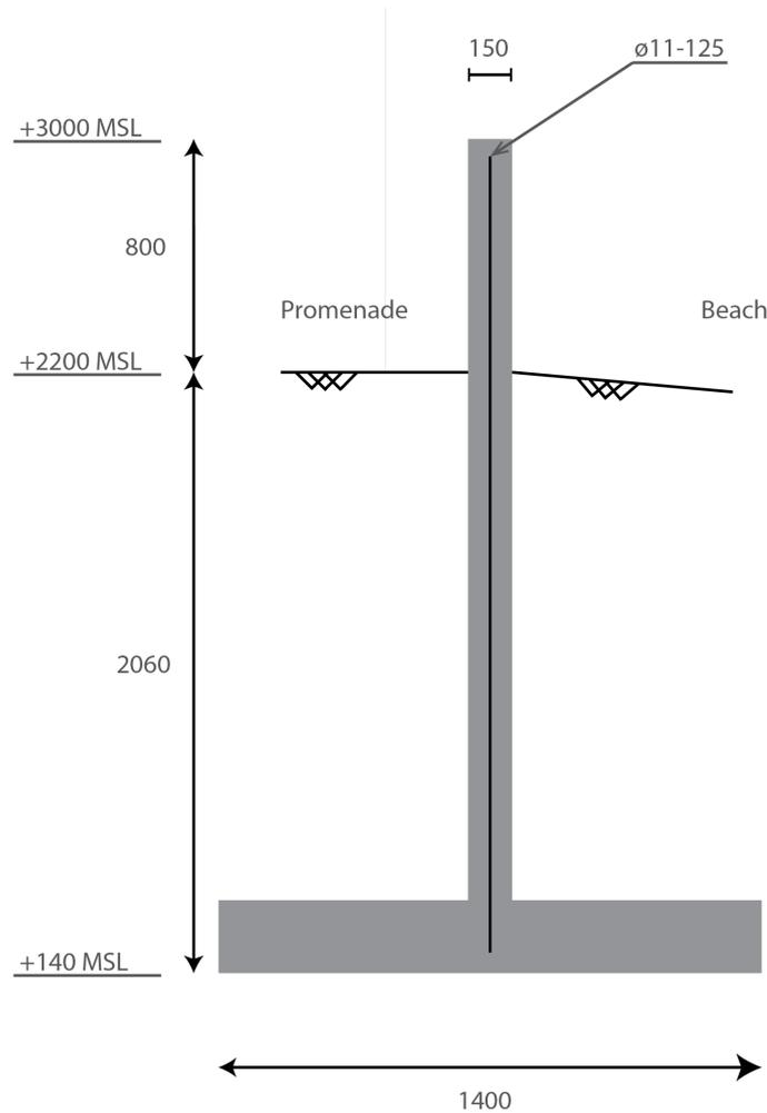
Figure 4.18: A section of the seawall, all measurements are in mm
