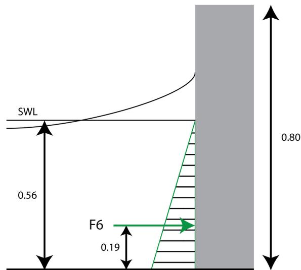
Figure 4.12: Hydrostatic pressure at the structure. Distances in meter.
