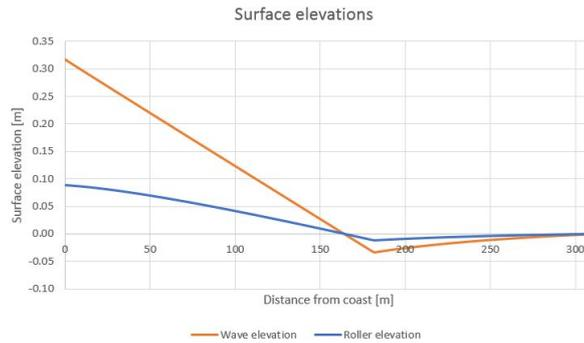
Figure J.3: Surface elevations due to wave set-up and rollers
