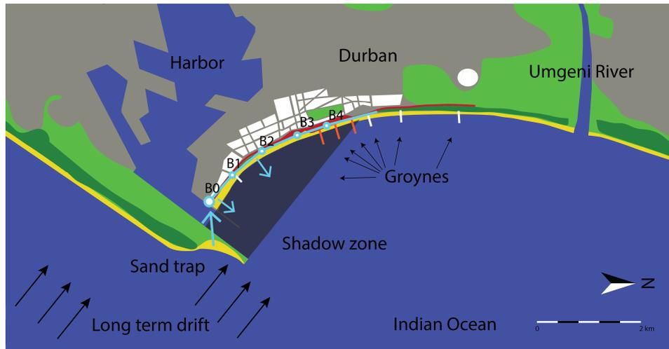
Figure 2.10: An overview of the considered area around the coast of Durban including sand pump scheme. Sand is trapped south of the harbour and pumped via various boosters (B0-B4) up north. Nourishment takes only place at the southern beaches while the pipe is constructed up north. Boosters 3 and 4 are not operational and nourishment of these beaches is done via offshore dredgers. The pumping scheme is shown more detailed in figure 2.11.
