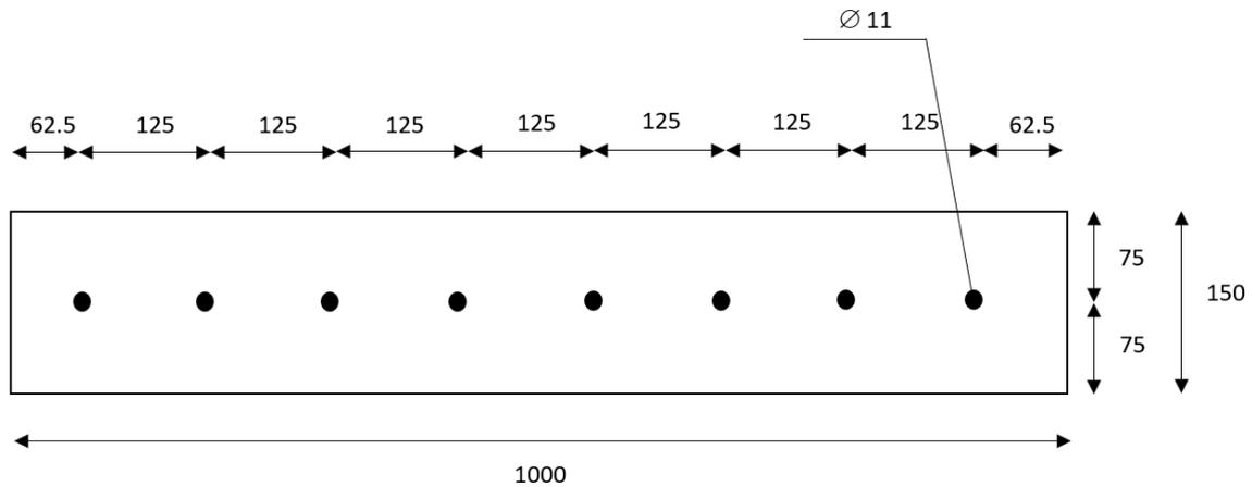
Figure 4.16: top view of the cross-section of the seawall, all measurements are in mm
