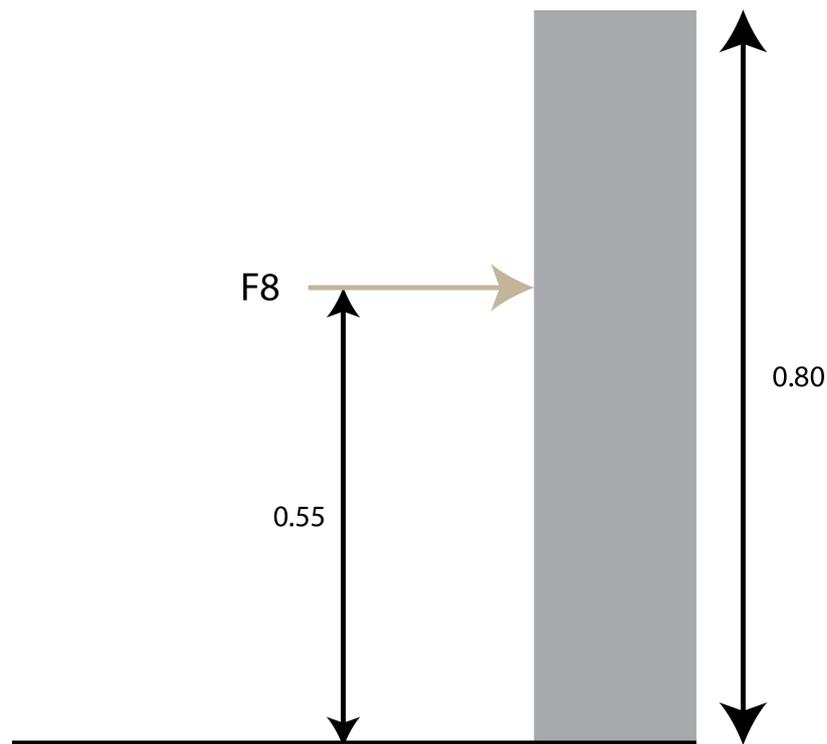
Figure 4.14: Horizontal forces acting on the sea wall due to accidental car impact. Distances in meter.
