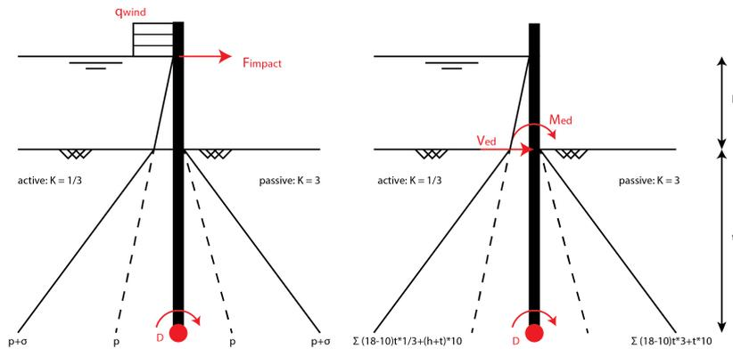
Figure L.4: Pressure diagrams as used for Blum's method for an infinitely stiff sea wall.
