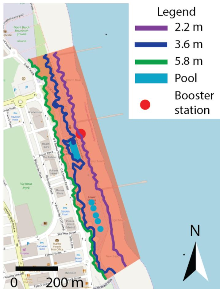
Figure 4.4: Obtained vulnerable area in red including elevation indication and booster location. Along this part of the promenade pools can be found as well.
