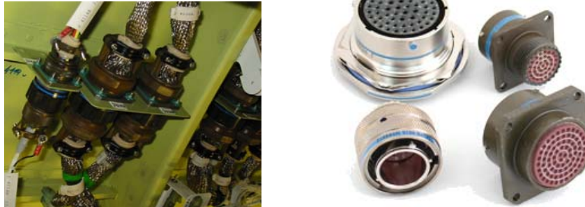
Figure 4: Connectors applied at a production break for electric wiring harness
