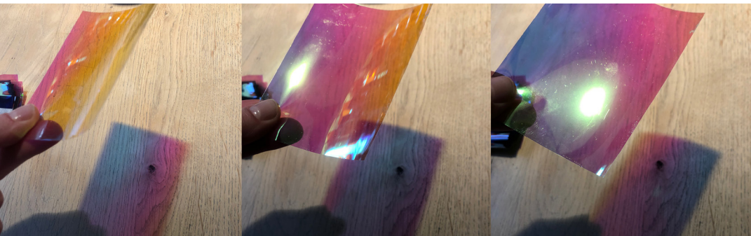
Fig. 58 - Showing the effect of a dichroic filter; leaving through other colors than seen on the paper (see shade) and reflecting green (see flash)
