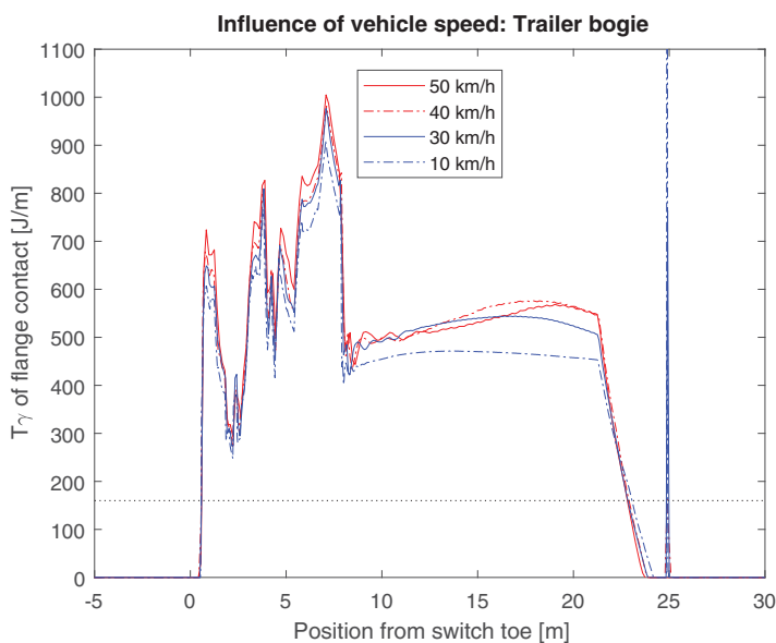
Figure 8. Wear loading for different train speeds. T_\gamma development at leading wheel of leading bogie.
