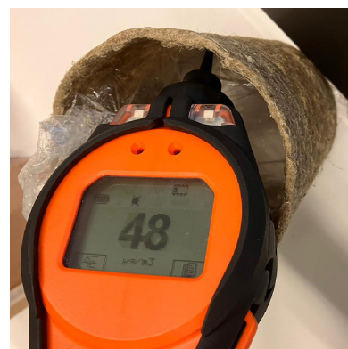
b) Measuring the chemical emission (VOCs), example bio-composite; flax fibre and bio-resin.
