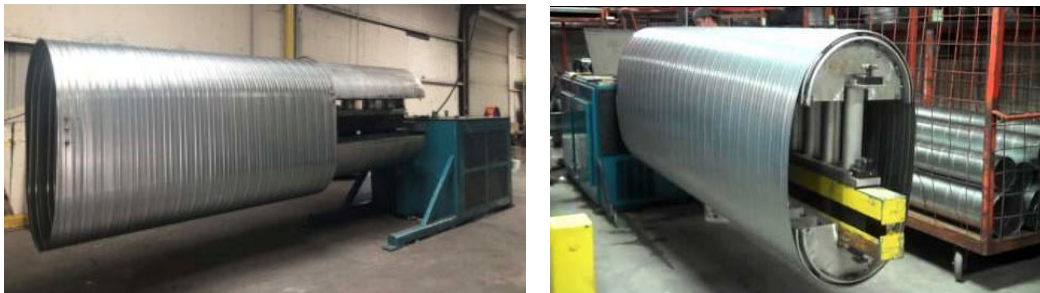
Figure 2.25 Stretching of spiral ducts to flat oval ducts (Spot, n.d.).
