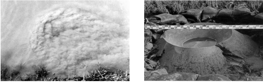
Figure 3.3: Sand boils: in action (left) and after flood event (right), courtesy of Rijkswaterstaat
