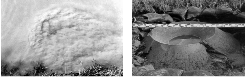
Figure 5.12: Sand boils (left: active during flood; right: post-flood crater; source: Rijkswaterstaat)
