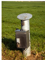
Figure 6.1: What you can see of an observation well at the surface.
