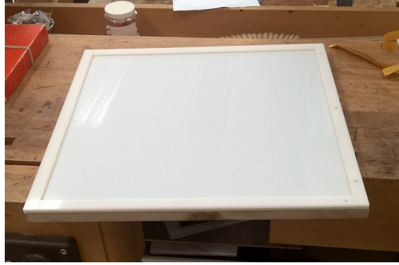
(b) Type II mould consisting of a MDF board backing and perspex surface, which is covered by a polyethylene film (not shown), adhered to the perspex with double sided tape. The inner dimensions are 0.49x0.49 m.
