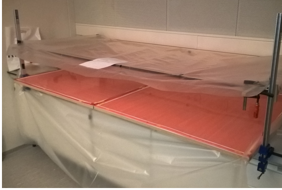
(a) Two type I moulds inside an isolated room at the Atelier Gebouw. An enclosure made from plastic film keeps dust from contaminating the gelatin solution.
