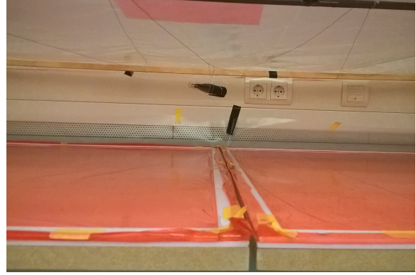
(b) Position of the Relative Humidity/Temperature-Logger inside the enclosure.
