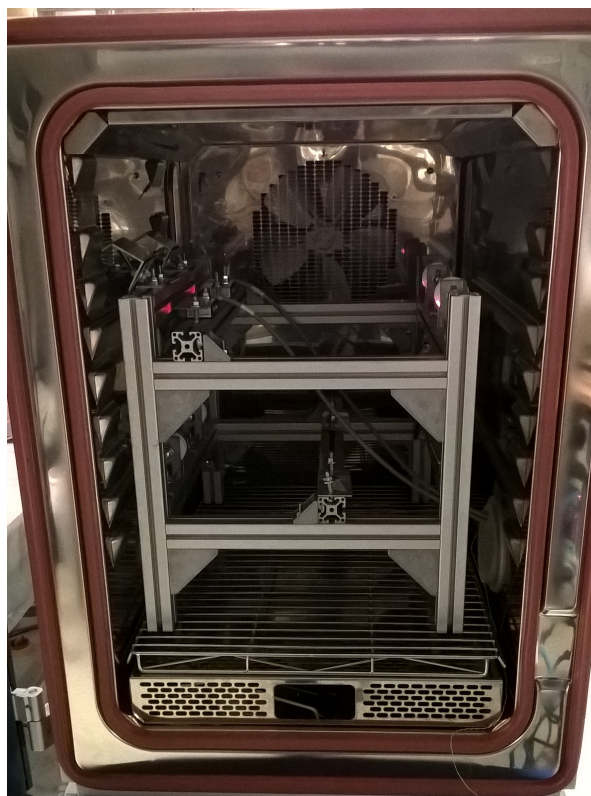
Figure 4.3: Creep bench in the climate chamber. The reflective surfaces are not present, as the samples are not yet mounted.
