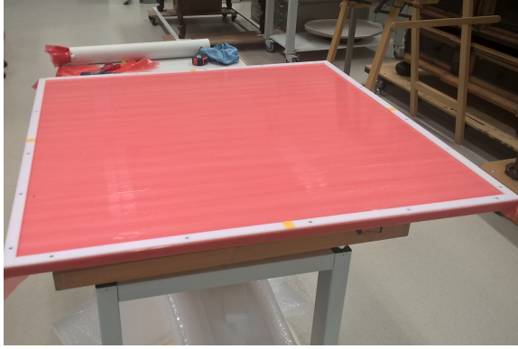
(a) Type I mould consisting of a MDF board backing and perspex surface, which is covered by a stretched teflon film acting as non-stick surface. The inner dimensions are 1.0x1.0 m.
