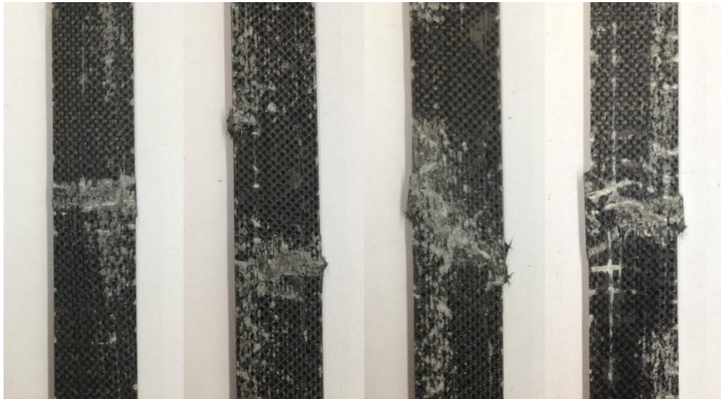
Figure 7.6: different failure modes in the 0° compressive test specimens
