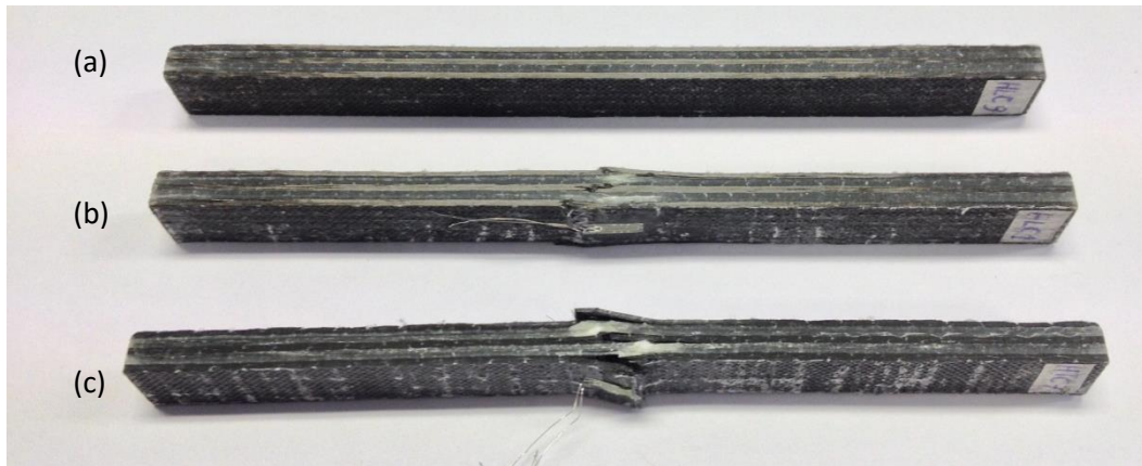
Figure 8.9: three hybrid compression test specimens: (a) before test, (b) 0° after test, and (c) 90° after test
