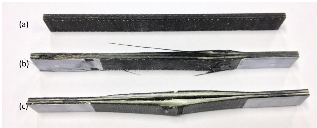
Figure 8.8: three hybrid tensile test specimens: (a) before test, (b) 0° after test, and (c) 90° after test
