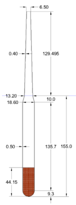
Figure 3.3: Illustration of the spar buoy platform WindCrete [32].
