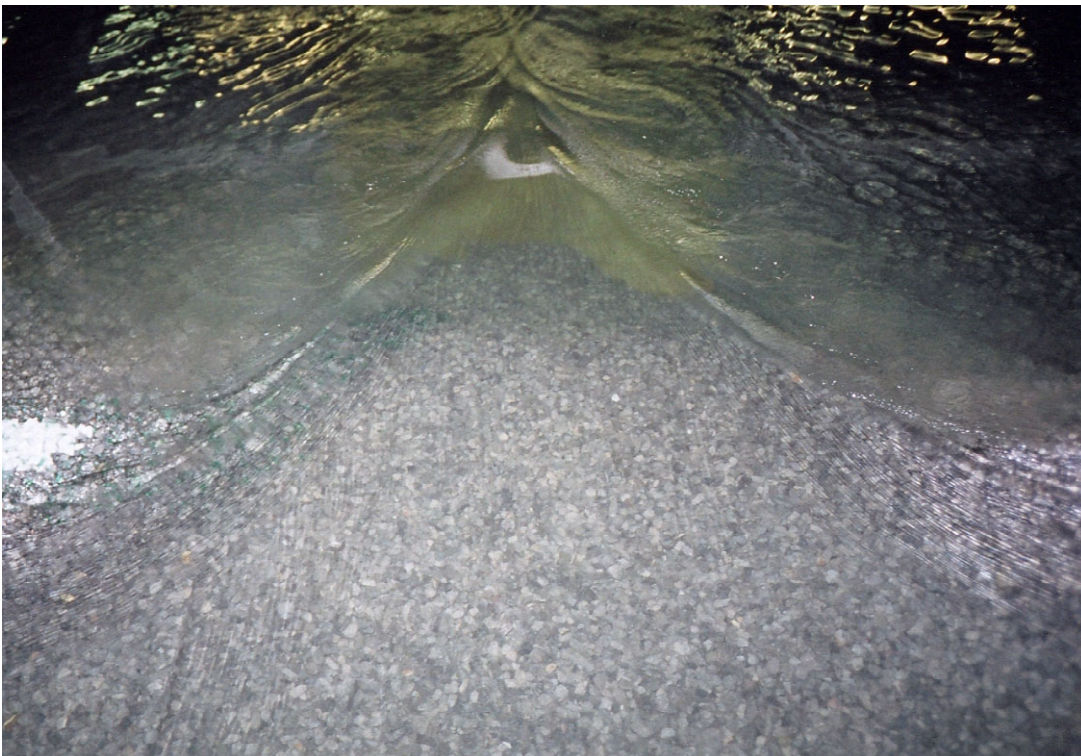
Plate 3.2 Flow contraction in closure gap
