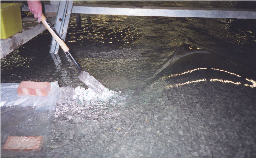
Plate 3.1 Simulated end dumping of single gabions
