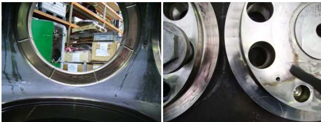
Figure 2.15: 4D1000 hub and blade carrier after 10 years service
