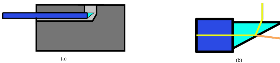
Figure 4.14: In (a), Solution C2-3. In (b), a detailed view of the tip of the fibre. The dark blue coating is removed leaving the optical fibre exposed. The tip is slanted to create a reflective surface. The yellow line represents the light reflecting and refracting.
