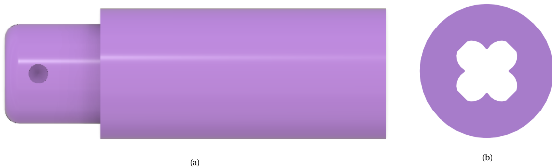
Figure 4.21: In (a), a top view of the prototypes body. In (b), the cross-section of the body. The clover-like shape will contain the fibre tubing.
