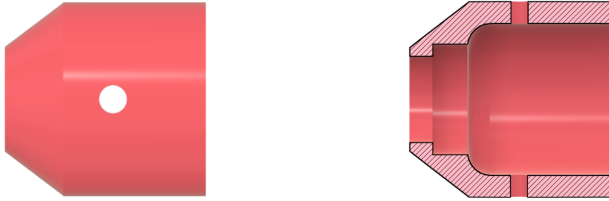
Figure 4.22: On the left, a top view of the connector. On the right, the cross-section of the connector. For the cross-sectional view, the connector was turned 90° to show the holes used for securing the connector to the body.
