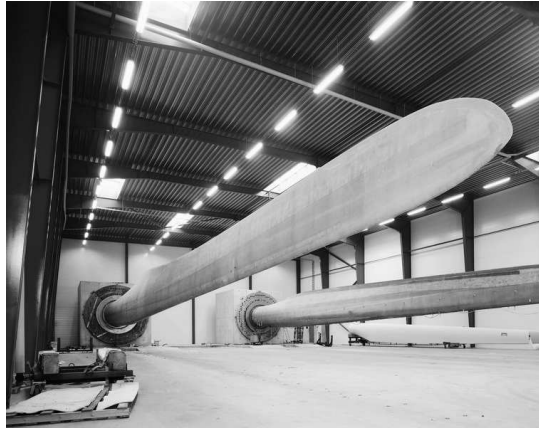
Figure 1.4: A wind turbine blade mounted to a test-jig. Courtesy of LM Wind Power.
