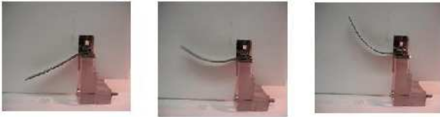
Figure 3.11: Motion of an IPMC under a low voltage
