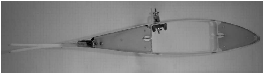
Figure 8.3: Overlay of two photo's of the actuator in maximum up and down deflection
