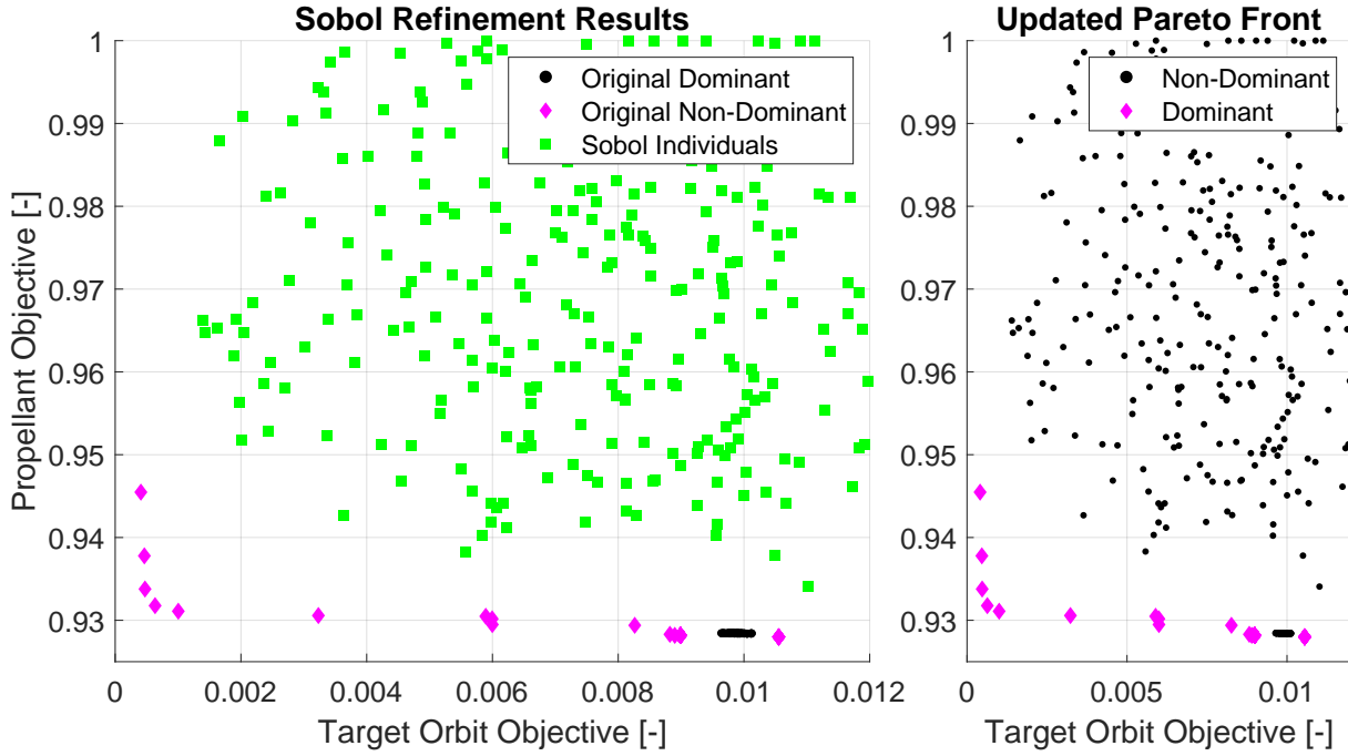
Figure 8.24: Pareto front with the Sobol analysis for an initial time of t_0 = 0 s.
