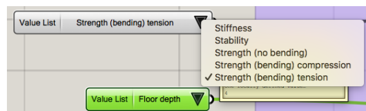
Figure 6.12: Feasibility checks offered by the tool, visualised in Rhino-Grasshopper
