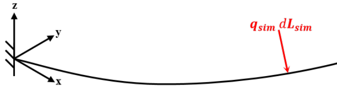
Figure 3.1: Lateral pressure force at a point on the cylinder in the global system, where q_{stm} is the distribution load. The cylinder is simplified to a curve for better illustration. The curve can be regarded as the central axis of the cylinder.
