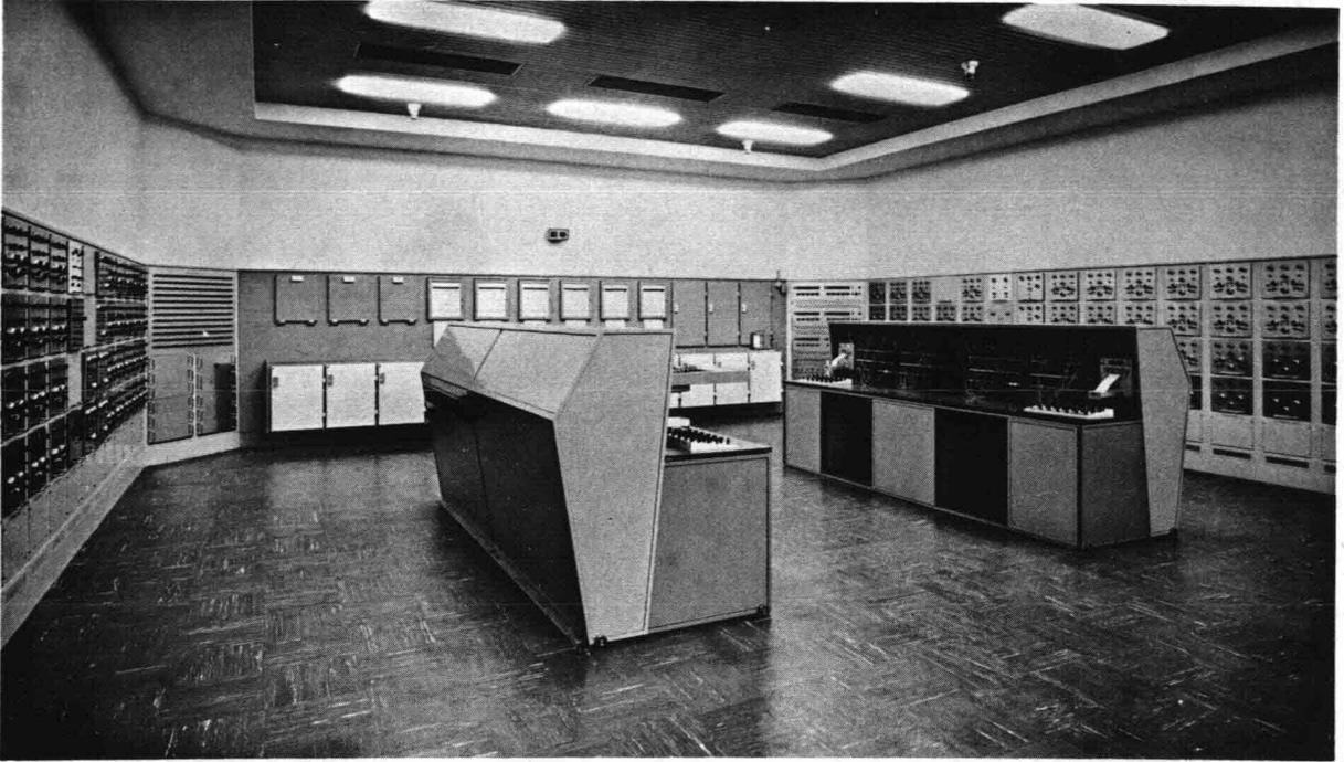
Fig. 1.7 DELTAR: analogue-digital model for the Netherlands' Delta (by courtesy of Rijkswaterstaat)
