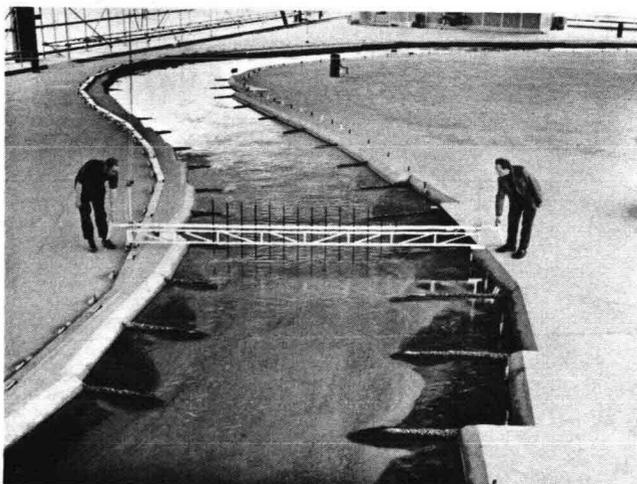
Also for morphological problems in rivers and coastal areas scale models are applied. In these cases watermovement and sediment-movement have to reproduced correctly to simulate bedlevel and bedlevel changes correctly.
