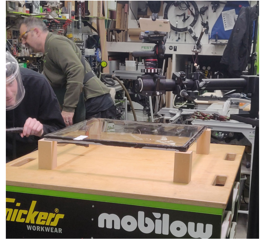
Inflation: Minimal pressure was needed to achieve a 10-15mm cavity
