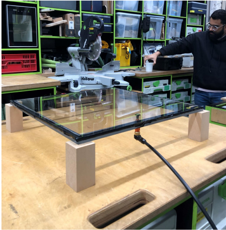
Setup: Unit on 4 wooden blocks with bicycle pump attached
