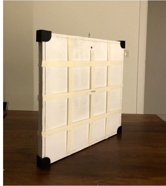
1.0mm Vivak 8mm deformation
