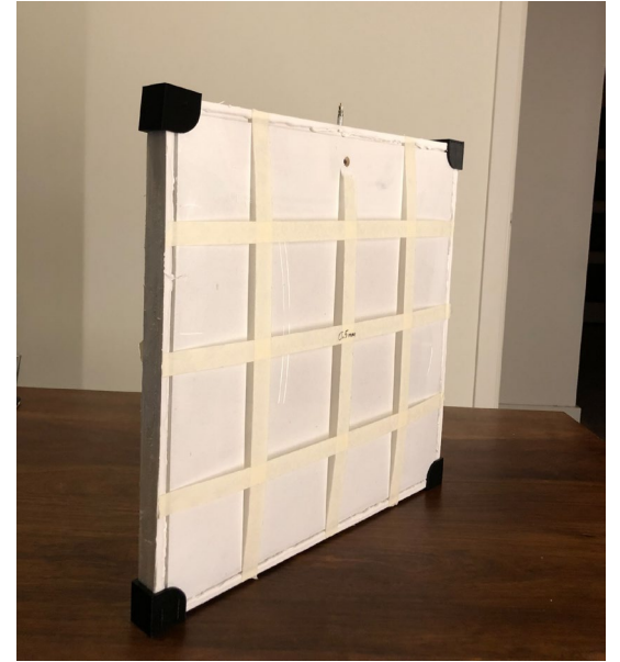
0.5mm Vivak 12mm deformation
