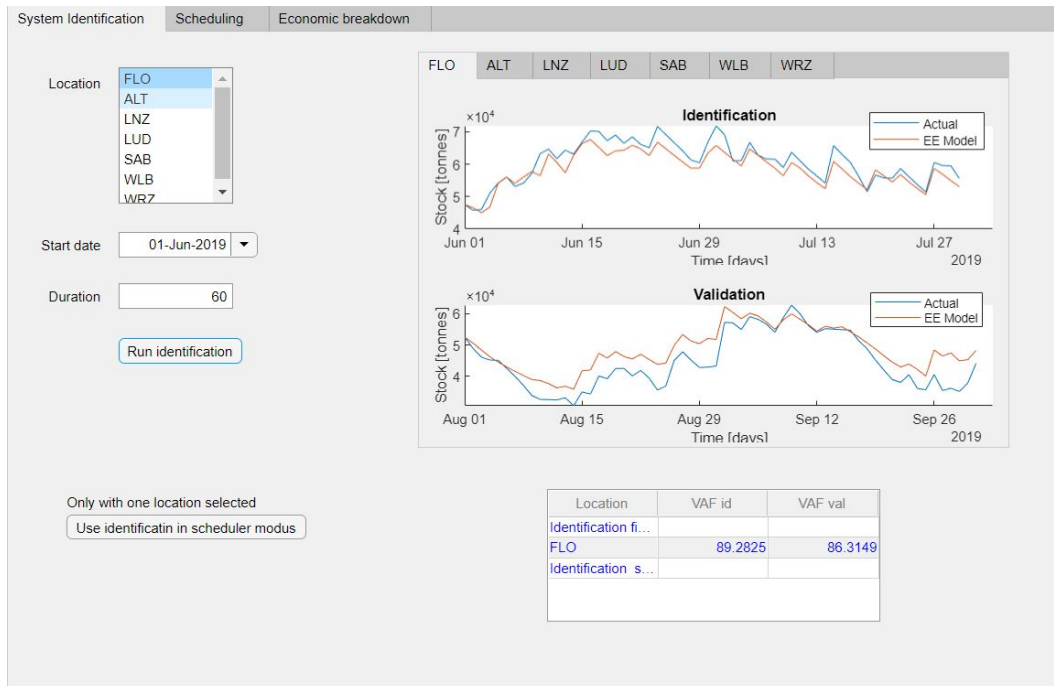
Figure 5-6: GUI tab for systems identification of the storage depot model for different locations.
