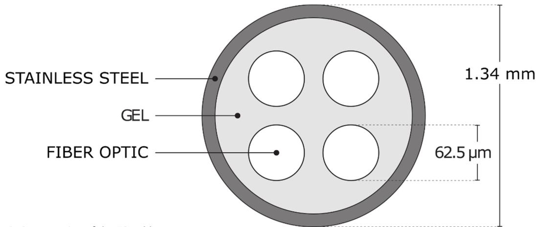
Figure 2: Cross-section of the FO cable
