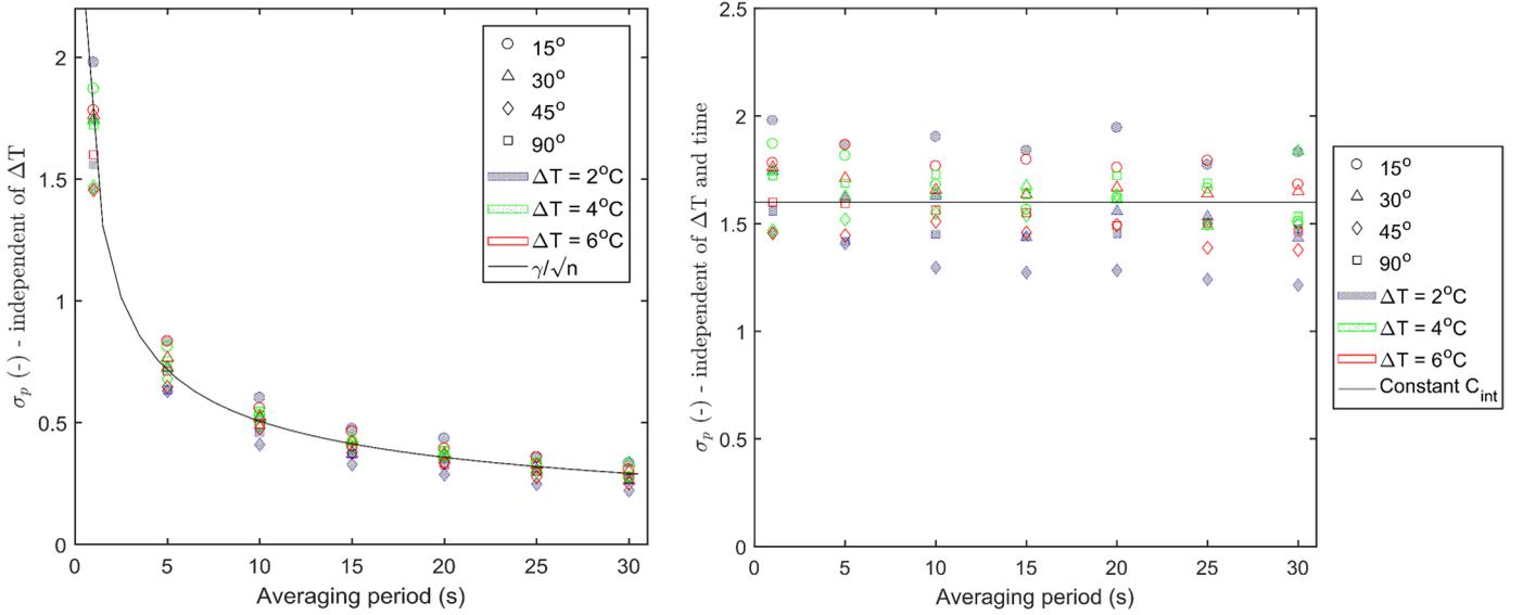
Figure 8 a) Precision of the AHFO wind speed measurements as a function of averaging period, independent of  $\Delta T$ ; and b) Precision of the AHFO wind speed measurements as a function of averaging period. Independent of  $\Delta T$  and averaging period.
