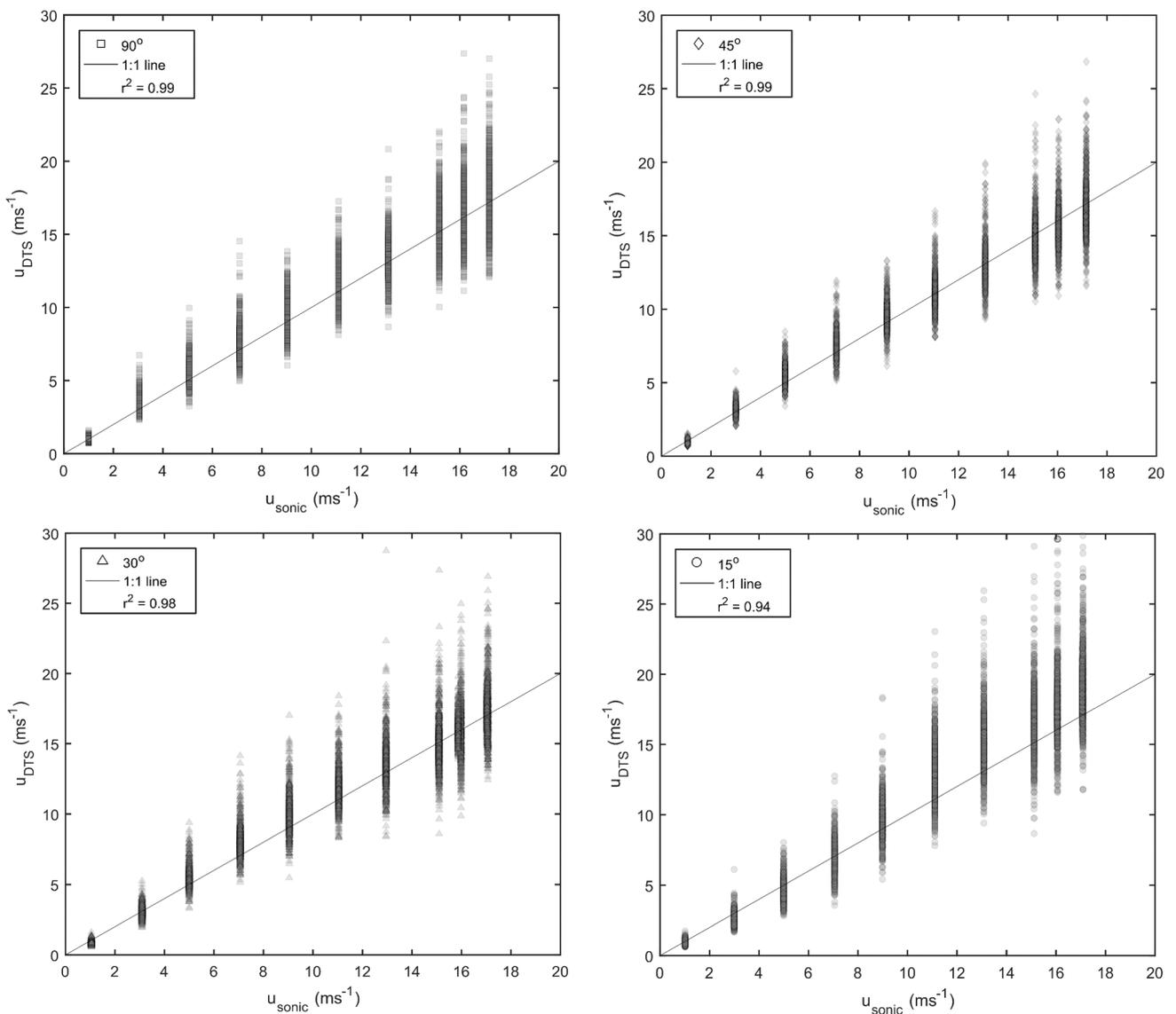
Figure 4a-d: Comparison of AHFO and sonic anemometer wind speed at a 1 s temporal resolution, for the four different angles of attack: a)  $90^\circ$ , b)  $45^\circ$ , c)  $30^\circ$ , and d)  $15^\circ$ .
