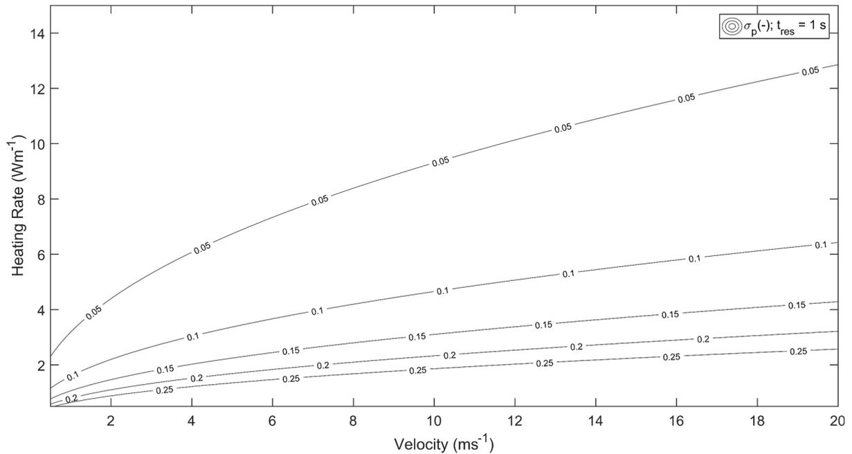
Figure 9: Expected error (contour lines) for a given heating rate and wind speed as calculated from Eq. 20, with a 1 s and 10 measurement resolution.
