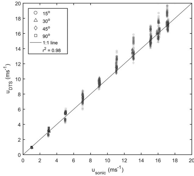
Figure 5: Comparison of AHFO and sonic anemometer wind speed averaged over 30 s for all angles of attack.
