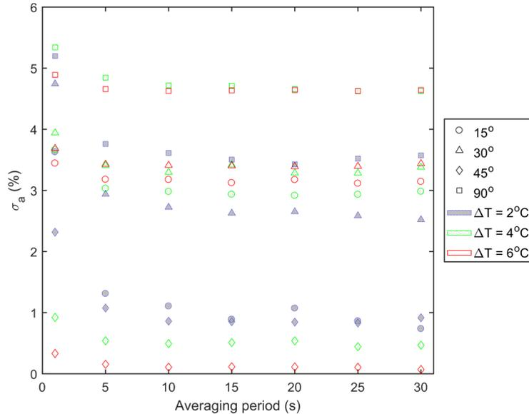
Figure 6: Bias in AHFO wind speed as a function of averaging period for different angles of attack, and different fiber heating.
