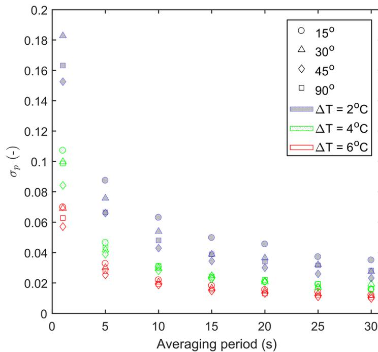
Figure 7: Precision of the AHFO wind speed measurements as a function of averaging period.
