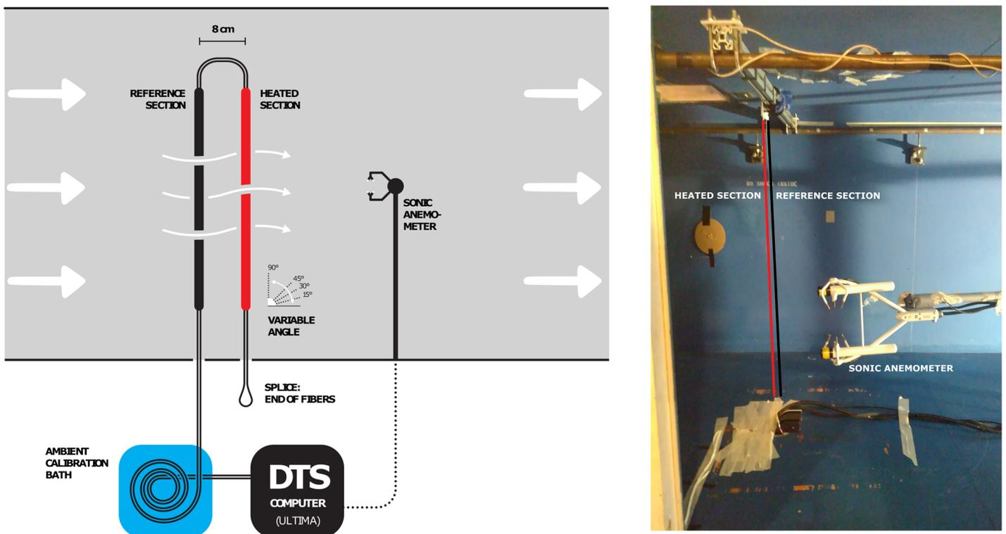
Figure 1 a) Schematic of the wind tunnel setup and b) photograph of the experimental setup in the wind tunnel.
