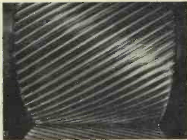
FIG. 7.—SCUFFED SECOND REDUCTION PINION (7/10-IN. DEEP TOOTH): ASTERN
