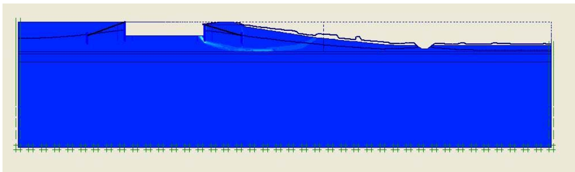
Figure 5.72: Deviatoric strain invariant distribution of failure mechanism following phase 3 of IM model
