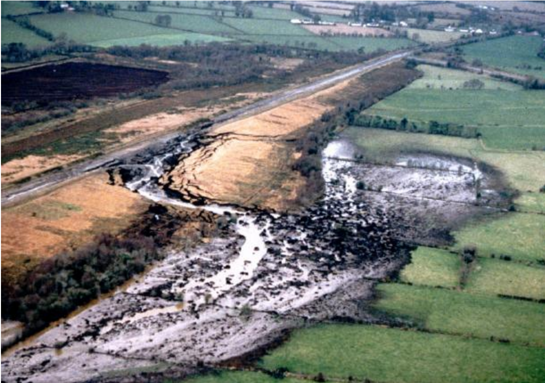
Figure 2.9: Aerial photograph of the Grand Canal breach in Edenburry, Ireland (Pigott, 1992 [13])
