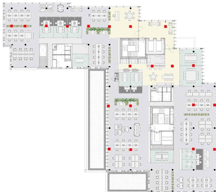
Figure 6.3: Floor Plan Concept 3 With Additional Columns
