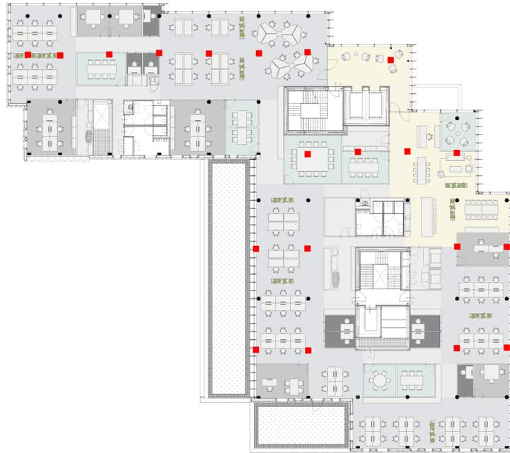
Figure 6.2: Floor Plan Concept 2 With Additional Columns
