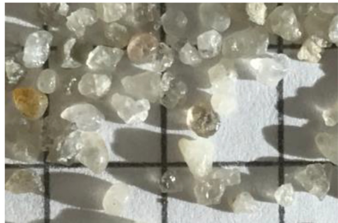
Fig. 2. Rapid sand filter granules 0.8 < d_p < 1.25 mm.
