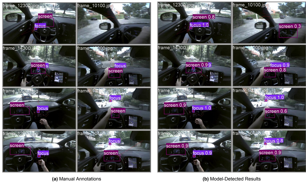
Figure 4.7: Testing Results for ADAS Brand A: (a) manually annotated bounding boxes and (b) YOLOv8-detected results
