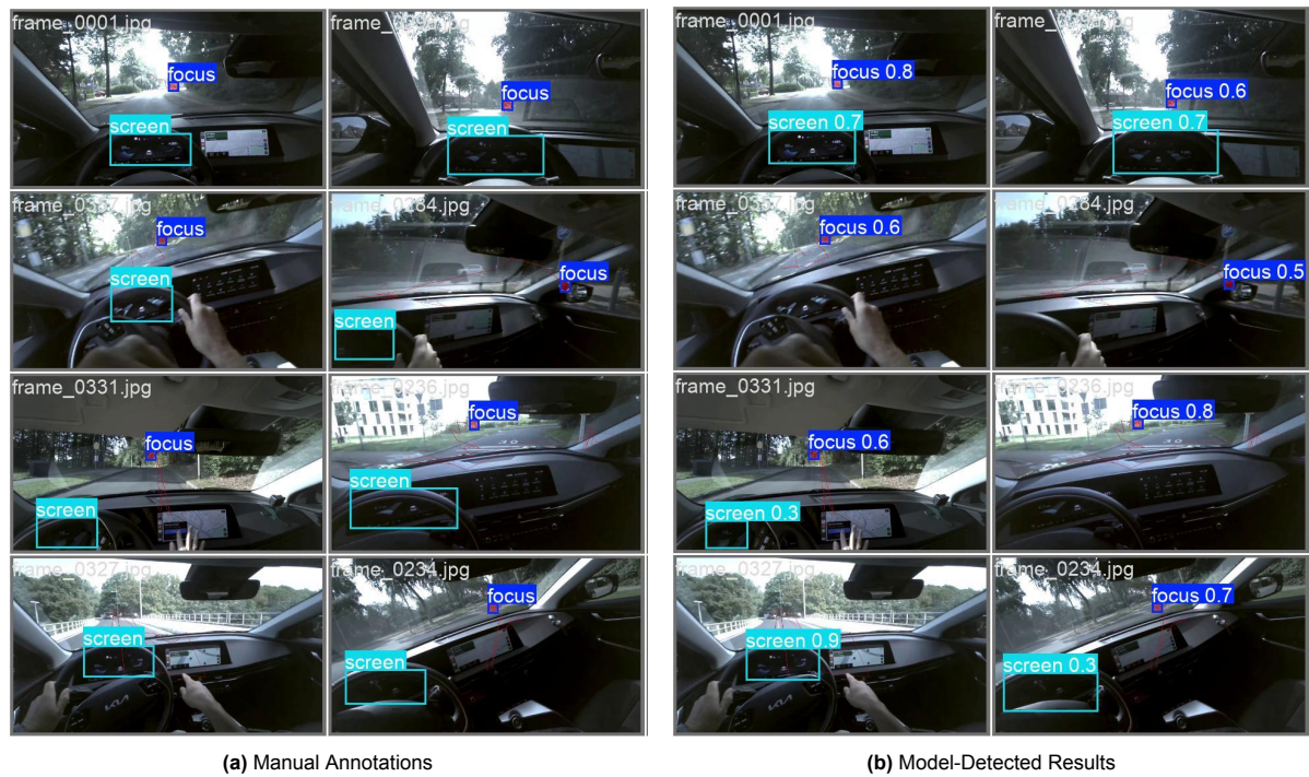
Figure 4.8: Testing Results for ADAS Brand B: (a) manually annotated bounding boxes and (b) YOLOv8-detected results
