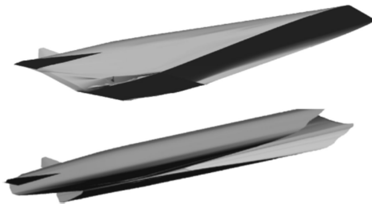
Figure 3.1: Illustration of a 2D scramjet and an inward 3D scramjet, taken from [22].
