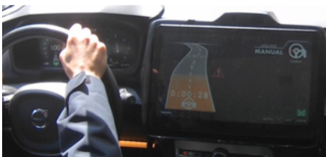
Fig. 6. HMI implemented in the prototype vehicle, showing the relevant time budget information derived from the proposed ASE, the LED bars show driving mode, as well as the remaining time budget by gradually shrinking.
