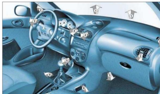
Figure 2 – View of the cabin car with all the vents highlighted. In the current experiments, only the vents indicated with 3 and 4 were open, whereas all the others were kept closed.
