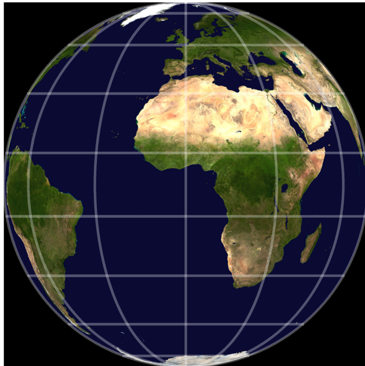
Figure 40: Orthographic projection. The equations are given by (3.3.1.1) and (3.3.1.2). Here, \phi_1 = 0 such that the center of the map corresponds to the coordinates (0, 0) on the sphere. The Orthographic projection corresponds to the Earth as viewed from infinity.
