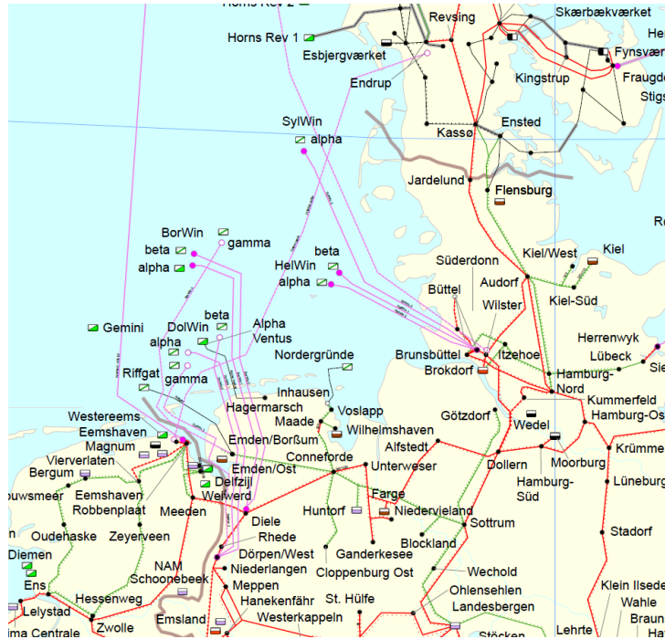
Figure 4.1. Map of the represented part of the European high voltage transmission network [55]
