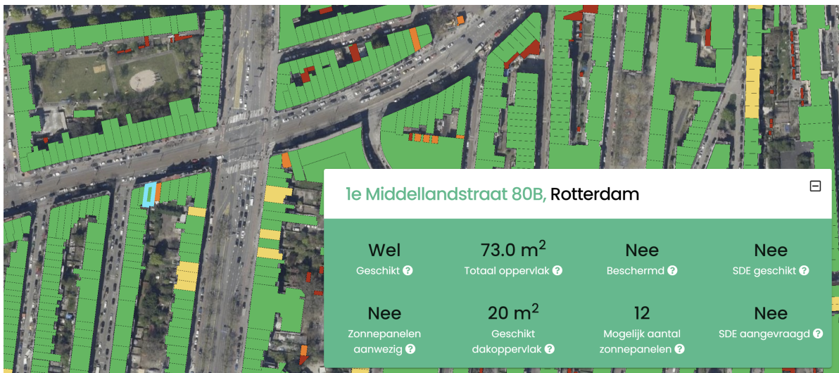
Figure 2.7: A Screenshot of the online Zonnedakje tool. Yellow indicates PV presence on a rooftop, red non-suitable roofs, orange possibly suitable roofs and green suitable roofs.
