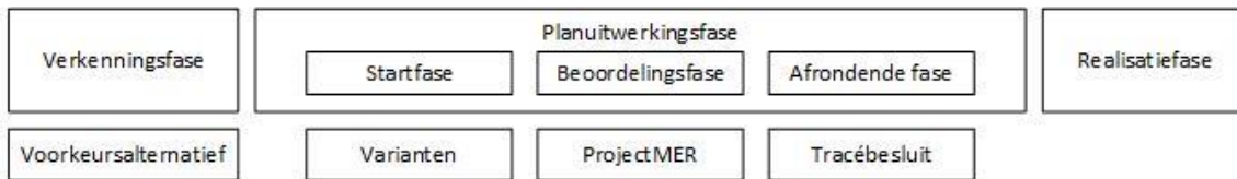
Figure 3.1: Visual representation of the planning process of the Planuitwerkingsfase. Simplification of system portrayed in RWS (2017, p.131) Left the first phase, Verkenningfase, middle the Planuitwerkingsfase and the last phase on the right.
