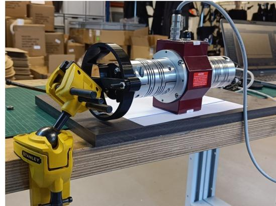
(d) The line drawn on the paper to check the alignment of the set-up is highlighted
