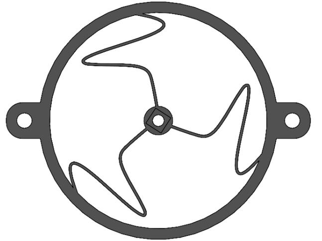
(b) Complete model of the joint with all the three flexures
