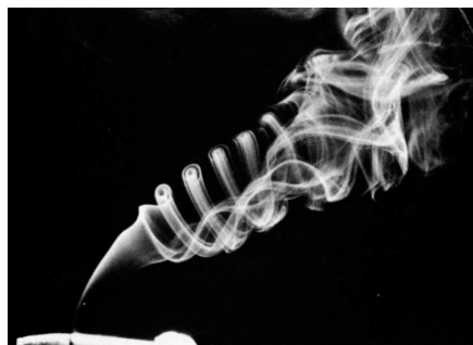
Fig. 1: Instability of smoke from a cigarette. The smoke rises vertically and smoothly for some distance (laminar flow) followed by transition into the turbulent regime due to growing undulations (taken from Van Dyke, 1988).
