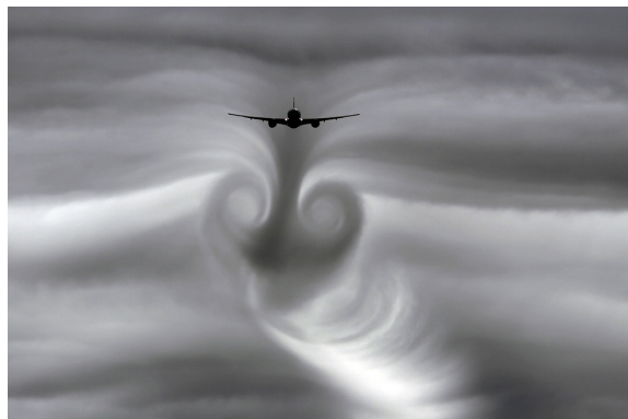
Fig. 3.16: Wing-tip vortices of descending aircraft visualized by clouds (with permission of Steve Morris; www.airliners.net ).
