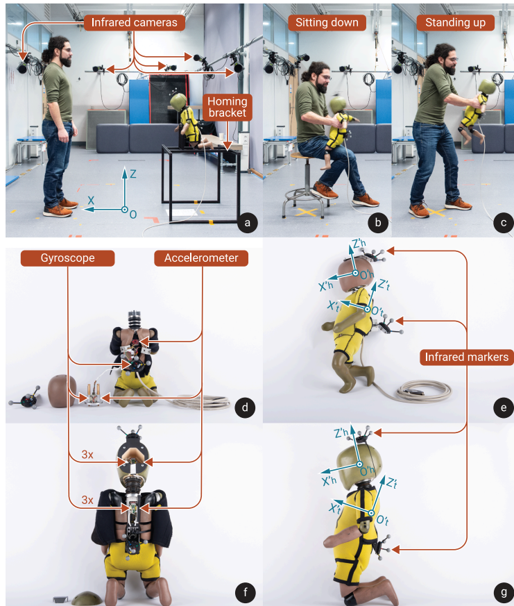
Figure 1. Overview of the experimental set-up and dummies used. The motion capture lab with infrared cameras used for tracking the dummy position, homing bracket that the dummy is placed in at the start and end of each trial, and global reference frame is shown (a). Two postures participants shook the dummy in were sitting down (b) and standing up (c). Accelerometers and gyroscopes integrated into Q0 (d) and Q1 (f) are indicated. The infrared markers used for tracking Q0 (e) and Q1 (g) are indicated, as well as their respective local head and torso reference frames.
